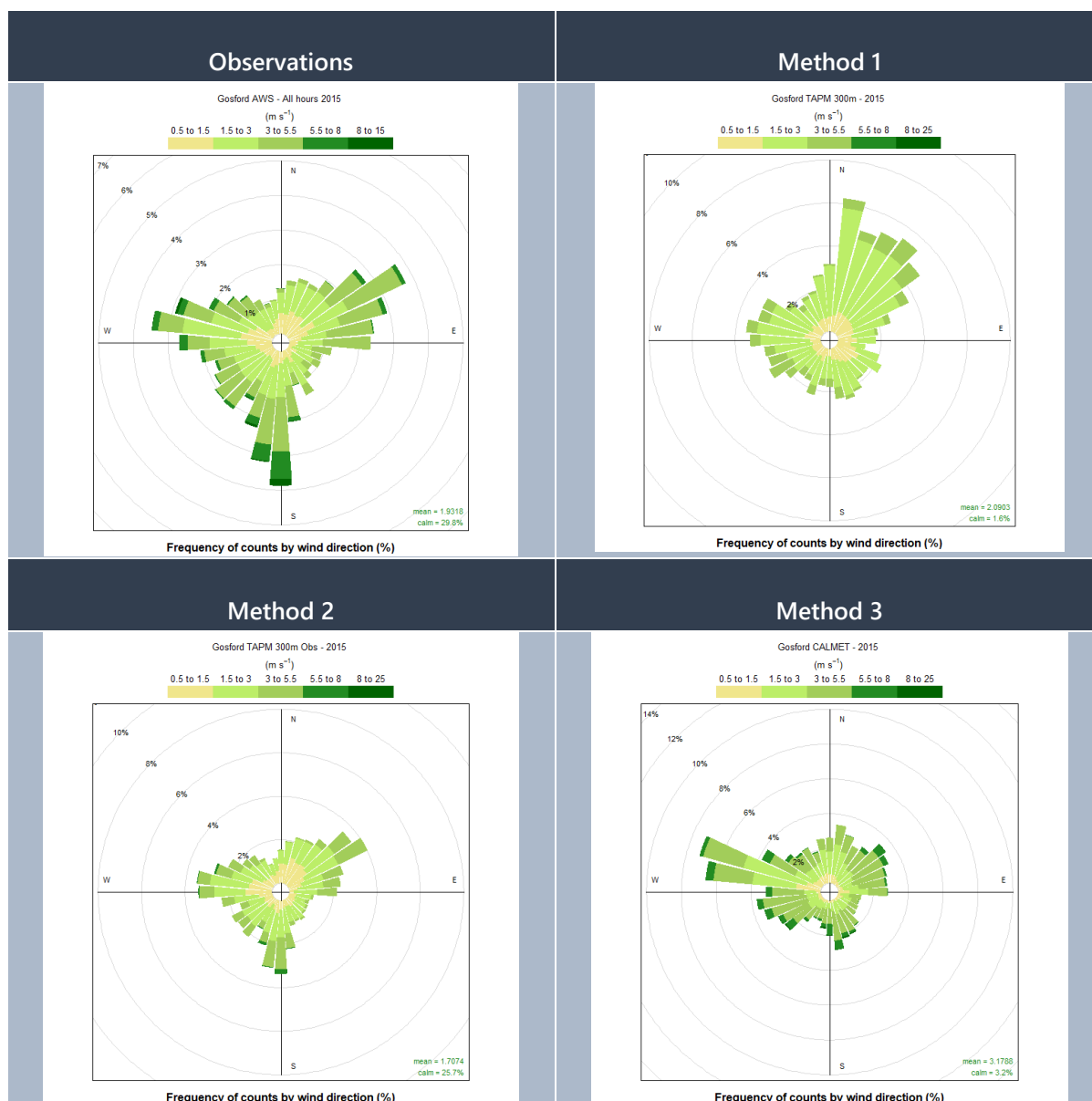
Figure 11 Observed and modelled wind roses – Gosford AWS 2015
