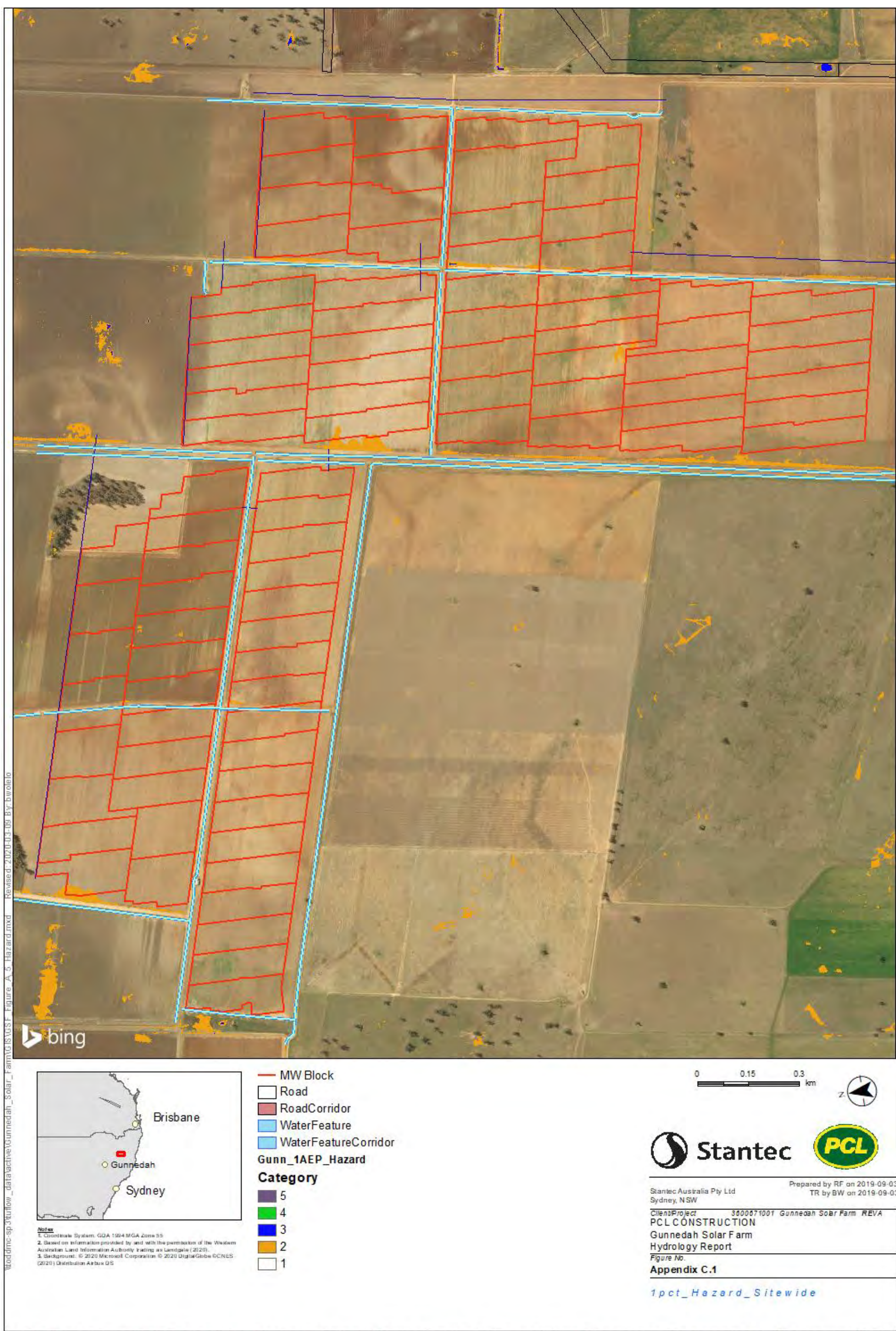
Figure Appendix C 1 Local overland Flow project site wide Hazard during the 1% AEP Storm event
