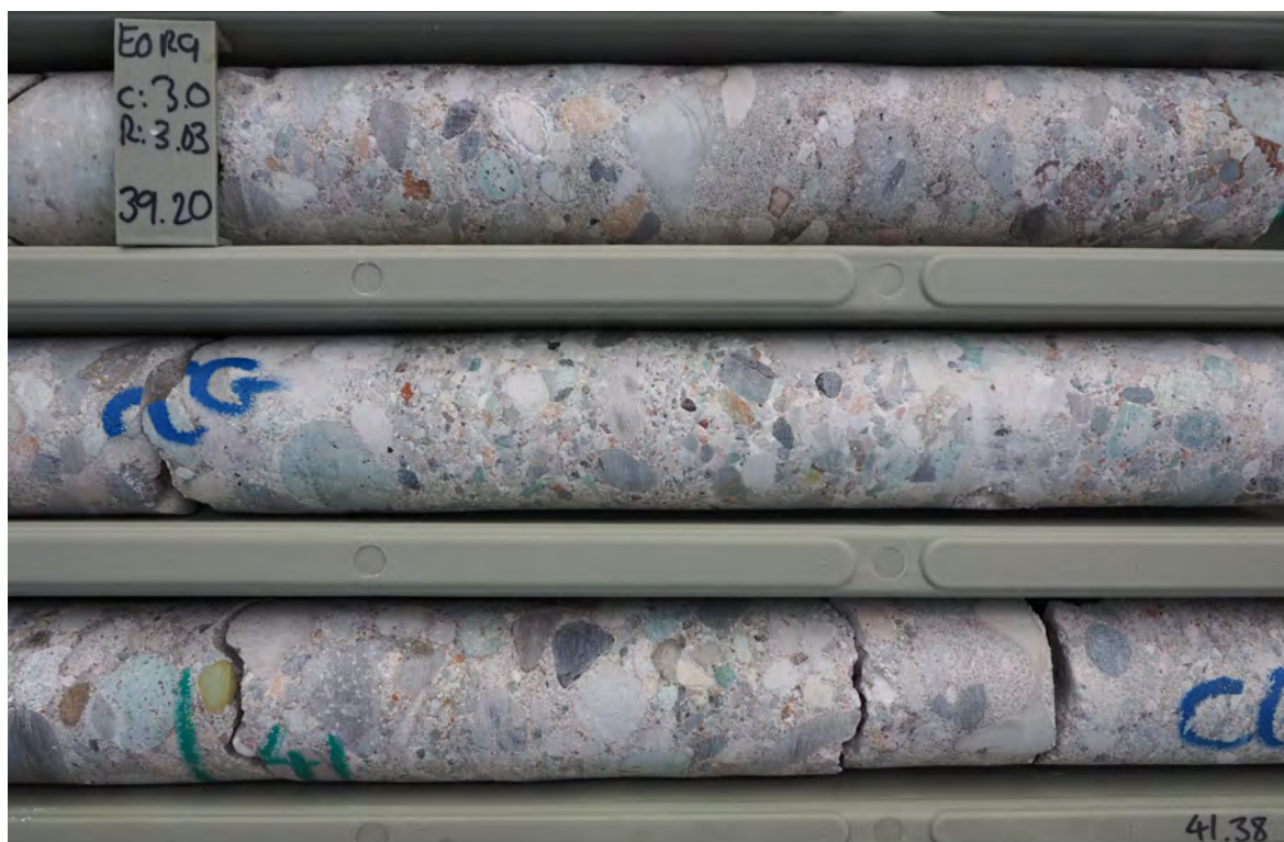
Plate 1: Typical conglomerate with no evidence of pyrite. Hole MN0003, between 39.0m and 41.4m.
