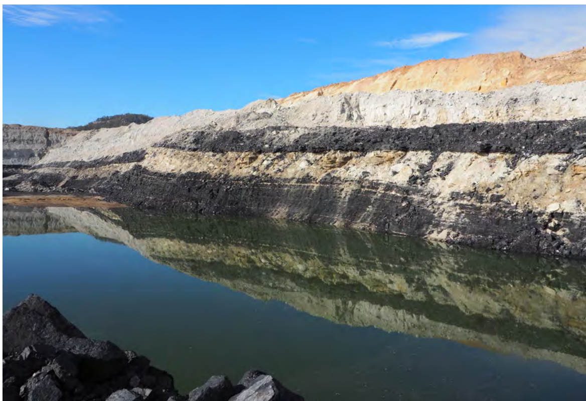
Plate 6: Exposed Great Northern and Fassifern Seam in Main Pit West Strip 8, showing no evidence of pyrite, pyrite oxidation or acid seepage from overburden/interburden or coal.
