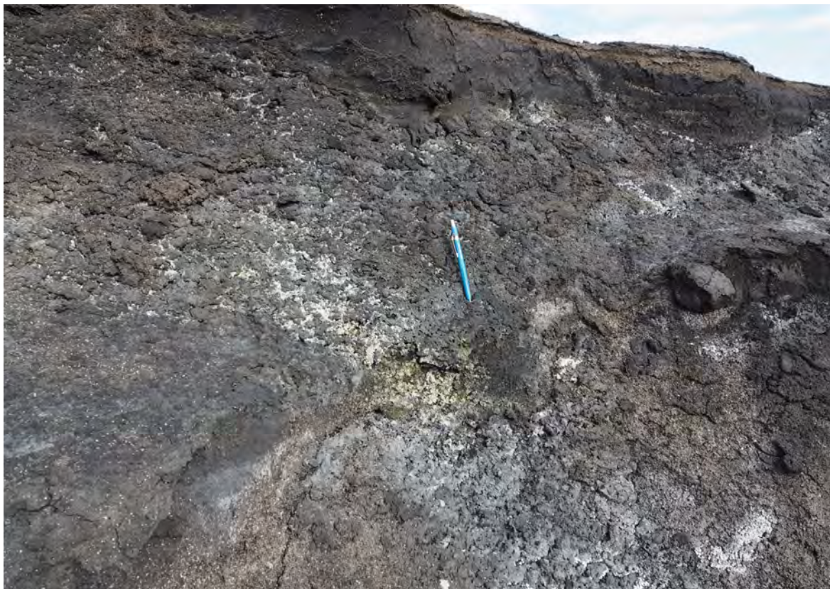
Plate 16: Tailings in the E corner of TD2 showing yellow and white salts typical of pyrite oxidation.
