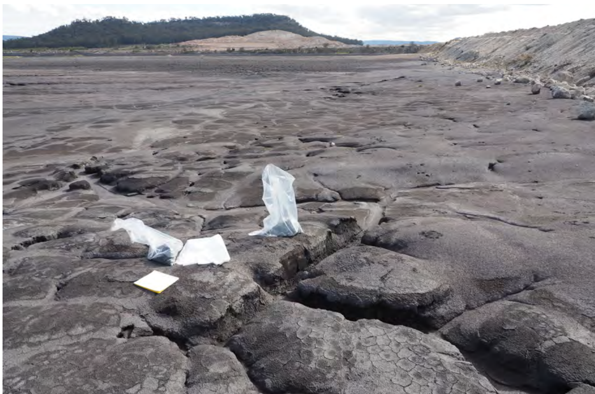
Plate 13: Tailings in the E corner of TD1 showing no evidence of pyrite or pyrite oxidation.
