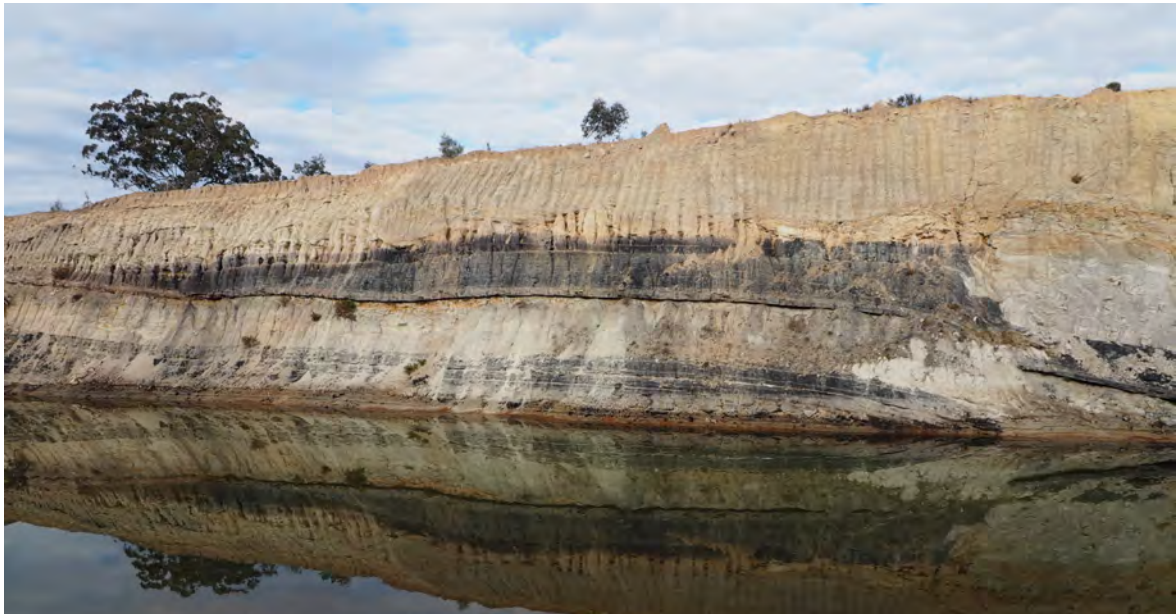
Plate 7: Exposed Great Northern Seam and Fassifern Seam in the original pit, showing no evidence of pyrite, pyrite oxidation or acid seepage from overburden/interburden or coal.
