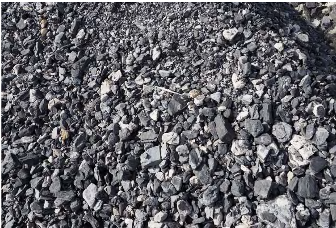
Plate 11: Coarse rejects co-disposed with overburden/interburden in South Pit showing no evidence of pyrite or pyrite oxidation.
