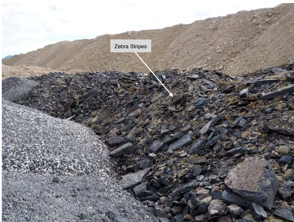
Plate 9: Zebra Stripes materials in Main Pit East, showing no evidence of pyrite or pyrite oxidation.
