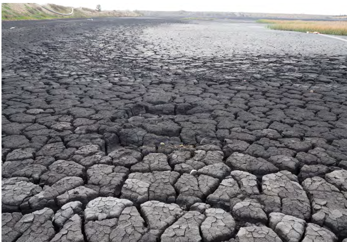
Plate 12: Tailings in the W corner of TD1 showing no evidence of pyrite or pyrite oxidation.
