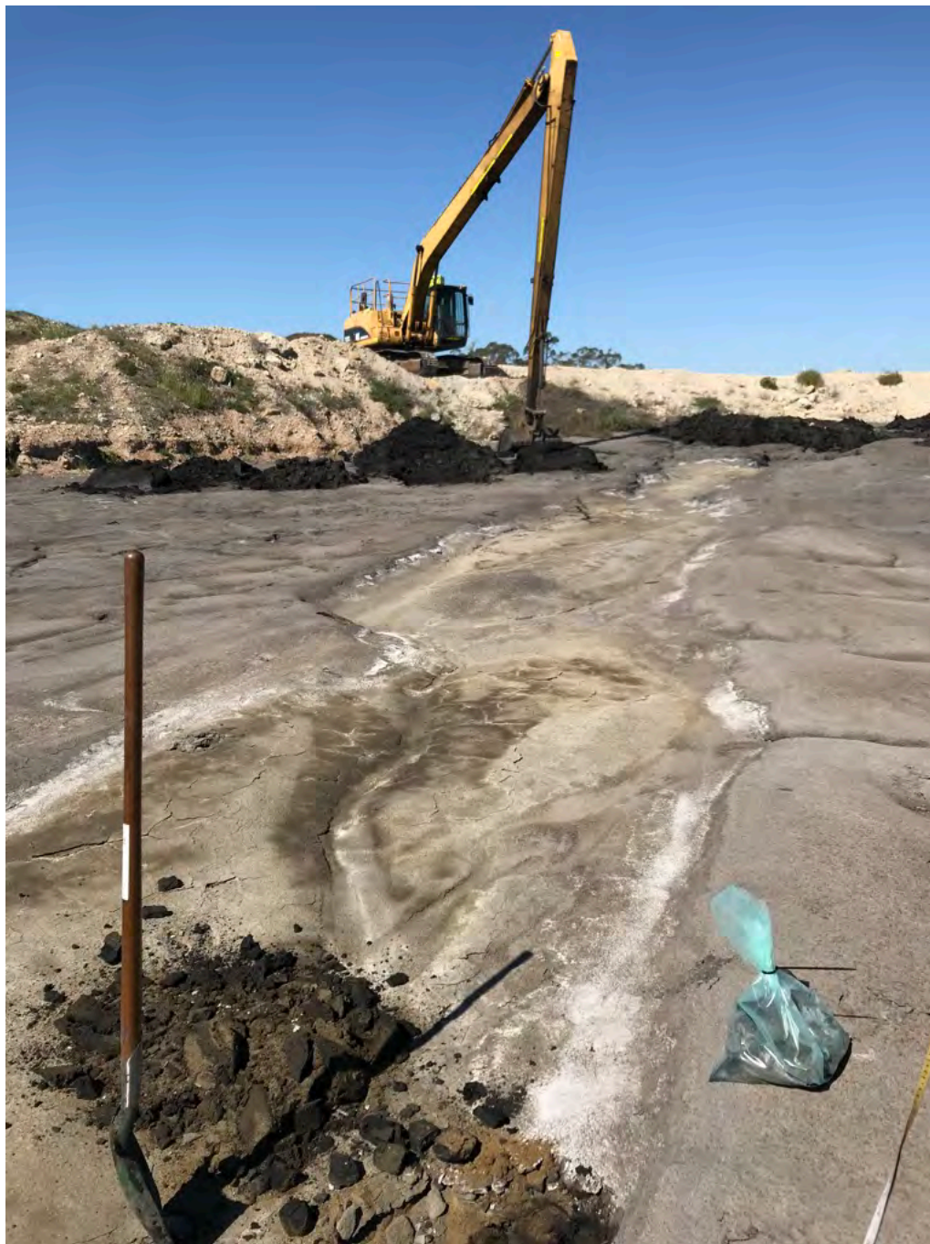
Plate 18: Long reach and hand shovel sampling at TD2 south corner.
