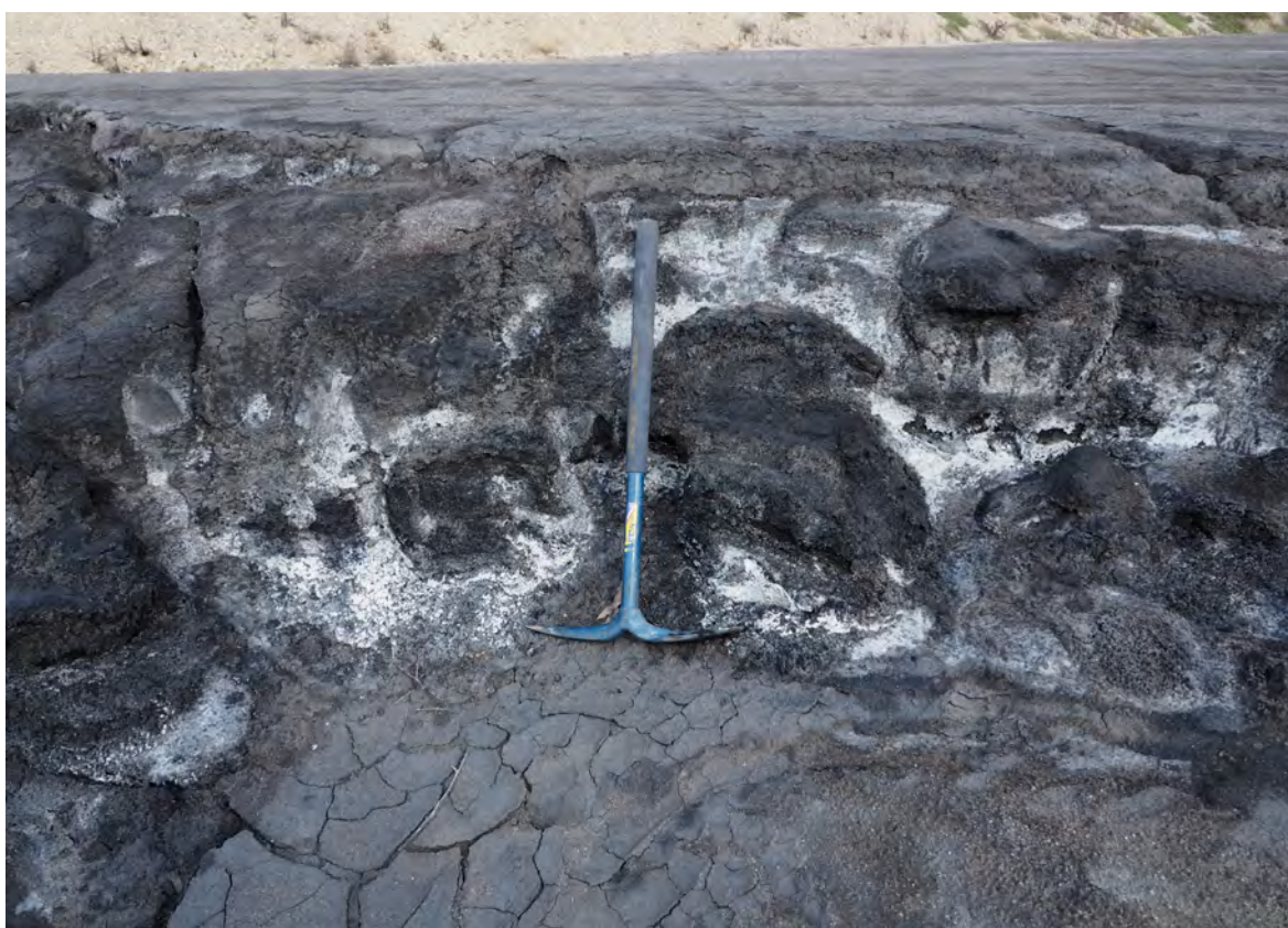
Plate 14: Tailings in the S corner of TD2 showing white sulphate salts typical of pyrite oxidation.
