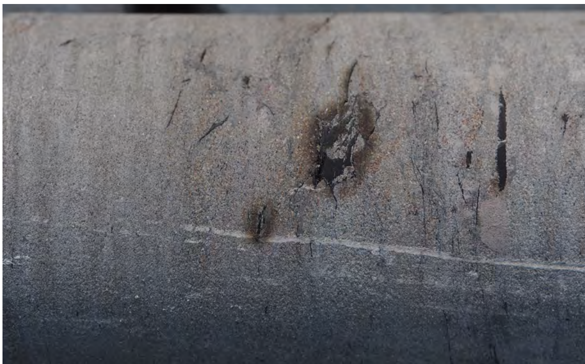
Plate 5: Iron staining after minor pyrite from coaly wisp in sandstone. Hole MN0003, 24.3m.
