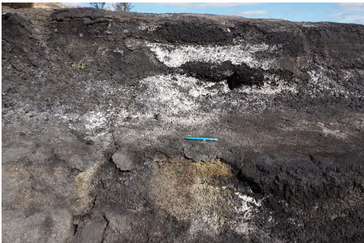
Plate 15: Tailings in the E corner of TD2 showing yellow and white salts typical of pyrite oxidation.
