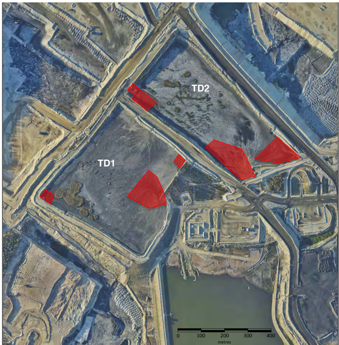
Figure 4: Plan showing areas of tailings sampling (as red shaded outlines) from TD1 and TD2.
