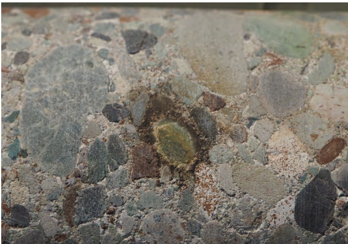
Plate 3: Iron staining and jarosite/sulphate salts after minor pyrite in conglomerate clast. Hole MN0001, 99.2m.
