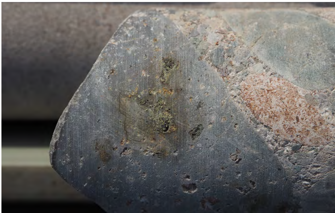
Plate 4: Jarosite/sulphate salts after minor pyrite in conglomerate clast. Hole MN0001, 98.5m.
