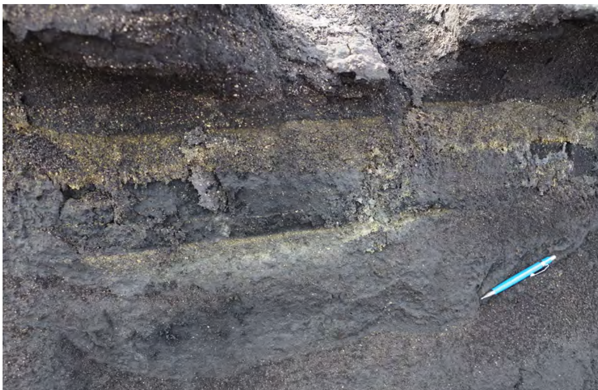
Plate 17: Tailings in the E corner of TD2 showing yellow and white salts typical of pyrite oxidation.
