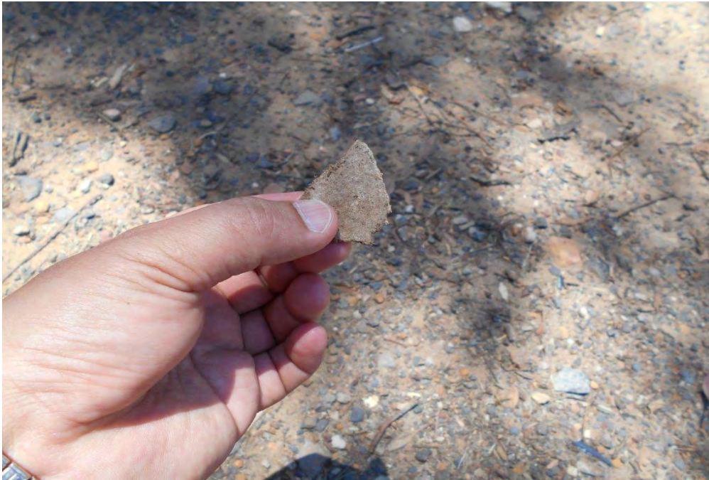
Photograph 5 - Fragment of PACM found on the ground surface near northern site boundary
