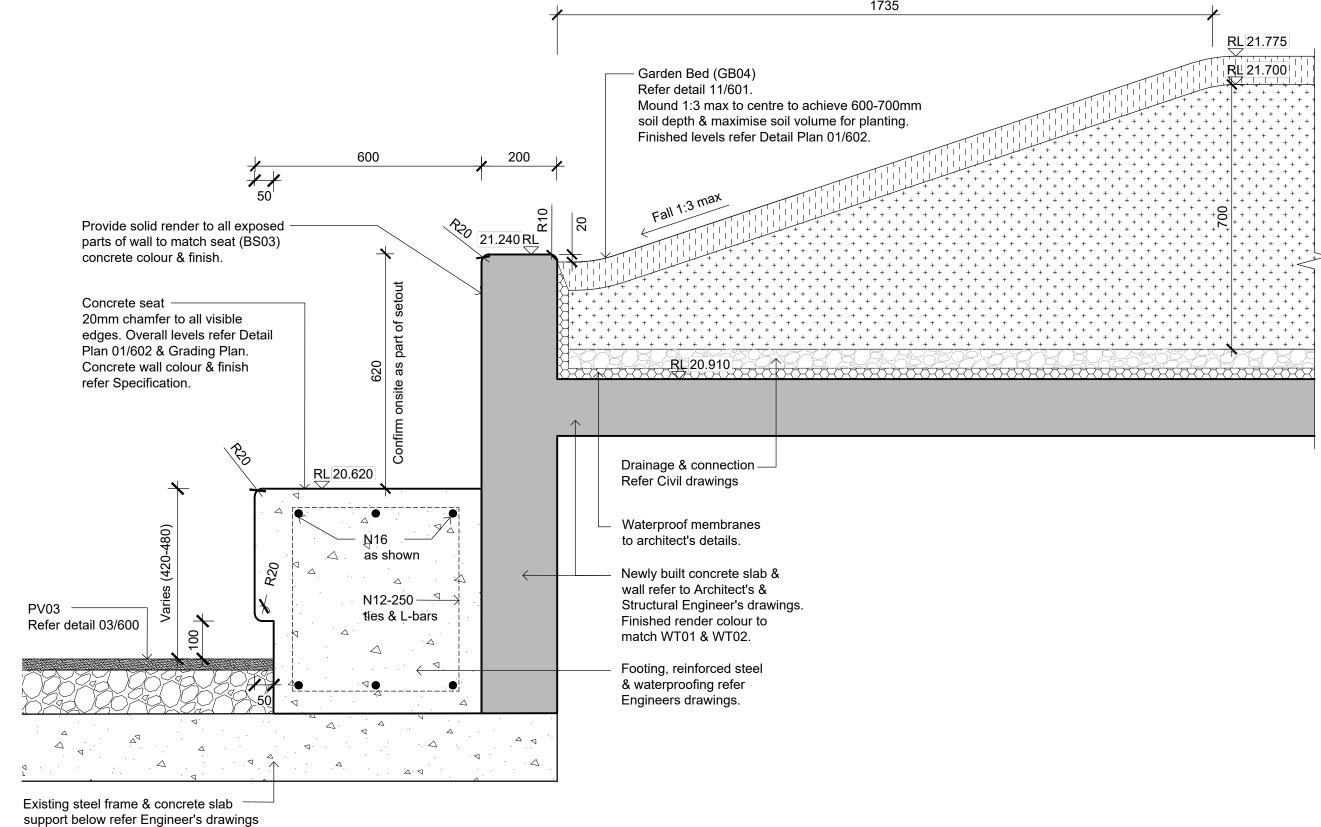
Garden Bed (GB04) -Refer detail 11/601. 21.240 RL 20.910 RL Refer detail 02/601 Refer detail 05/601. Raised edging 50mm above the finished lawn surface. Fall 1:3 may Newly built concrete slab & – SL01 (Lawn) Refer detail 01/601 wall refer to Architect's & Structural Engineer's drawings. Finished render colour to DANGAR LI MANNA MANANGAR MANAKA M match WT01 & WT02. Waterproofing refer Engineers drawings.
