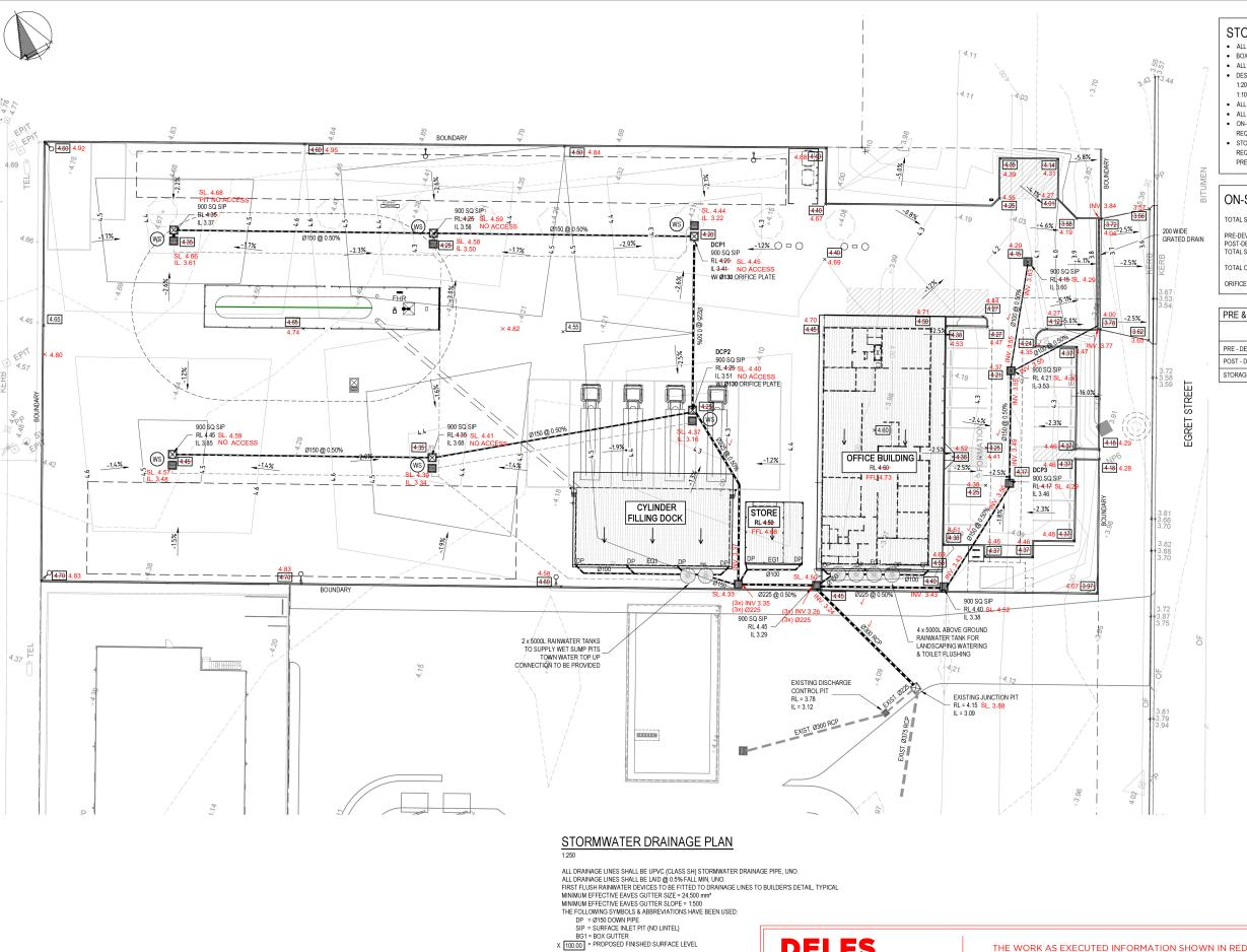
WS = DENOTES WET SUMP PIT - REFER TO TYPICAL DETAIL ---- = DENOTES WATER SUPPLY PIPE TO WET SUMP PITS
