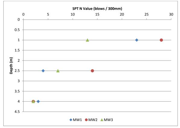
The standard penetration test (SPT) results are shown on Figure 2.
