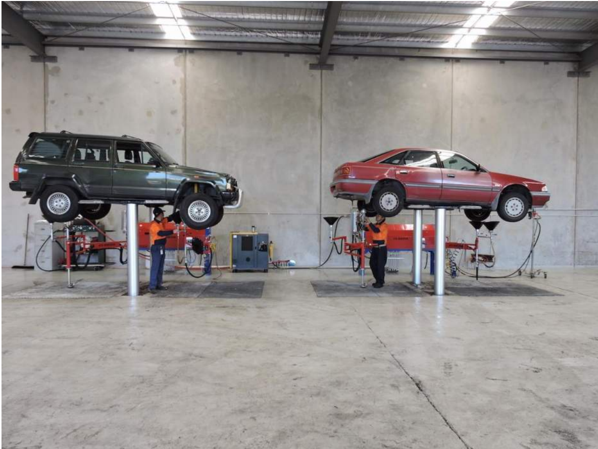
Figure 9: SEDA Easy Drain System - typical workstation with hydraulic hoist
