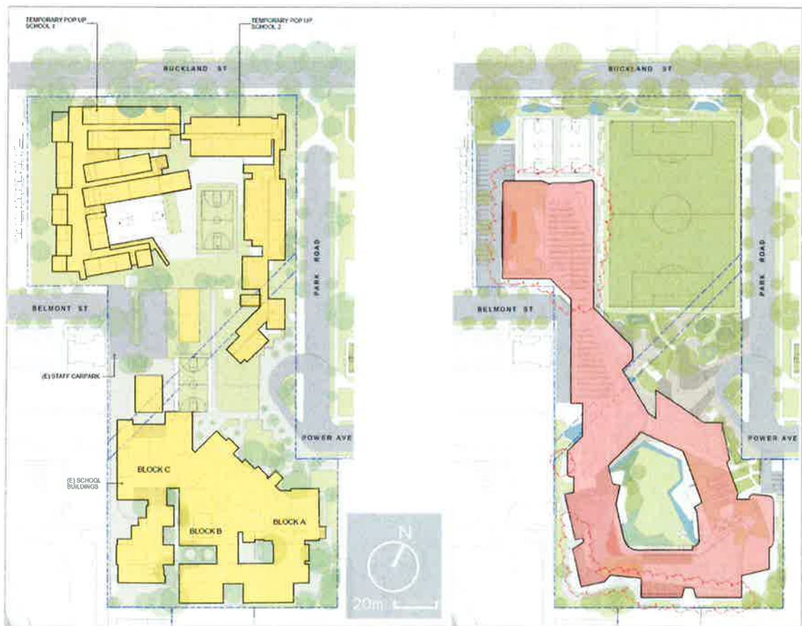
Figure 9 | Phase 3 Demolition and construction of outdoor sports field and entry forecourt (Source: Applicant's RtS 2018).
