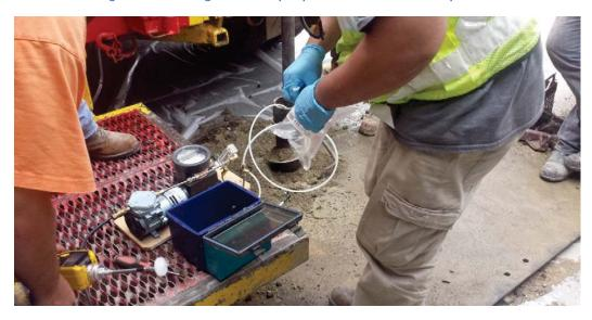
Figure 3 - A sample in a Tedlar bag is retrieved and ready to take a reading from using a PID meter (lower left).
