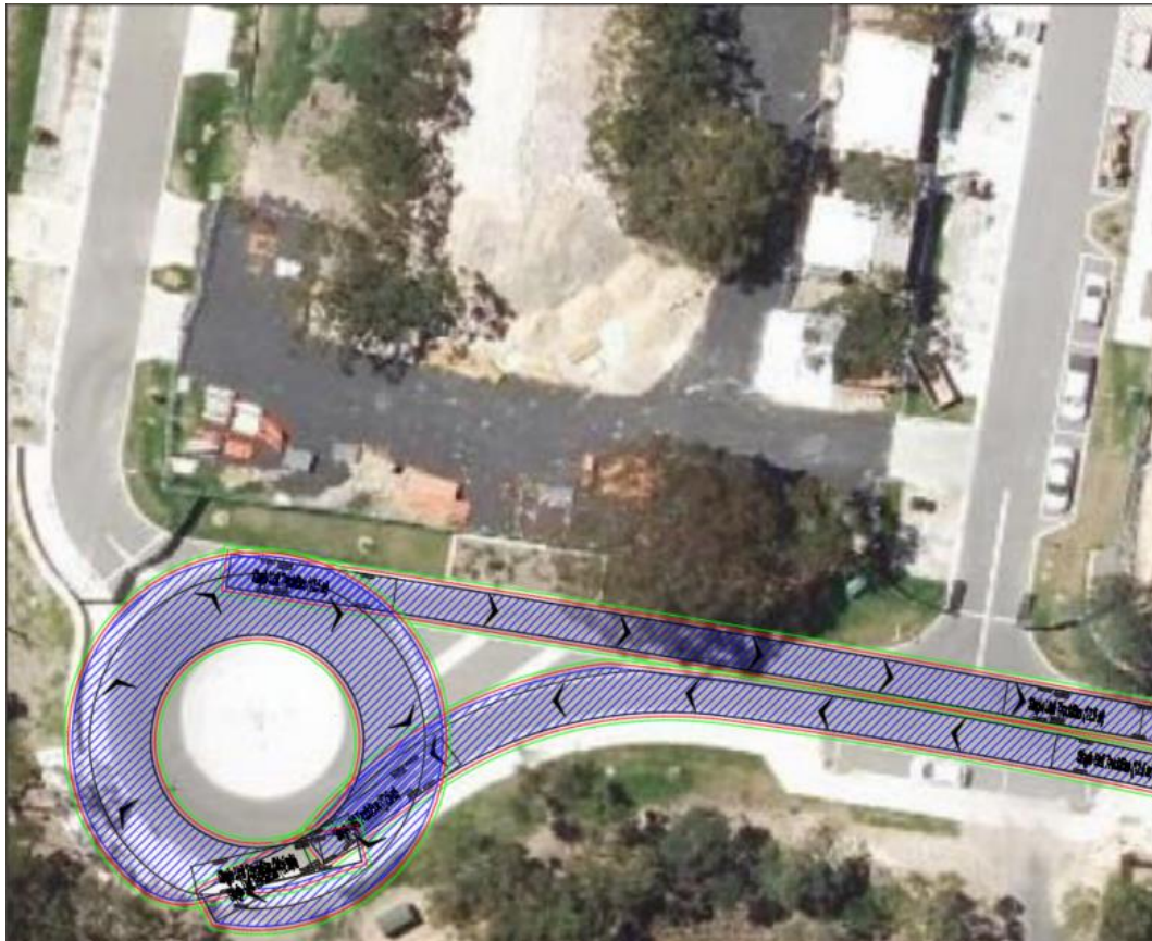
Figure 12: Utilising existing roundabout option, 12.5 metre bus
