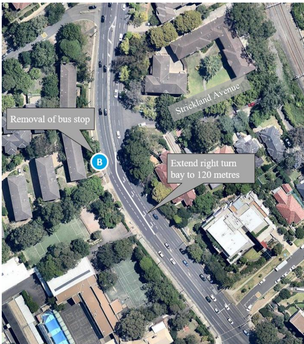
Figure 22: Schematic of proposed upgrades
