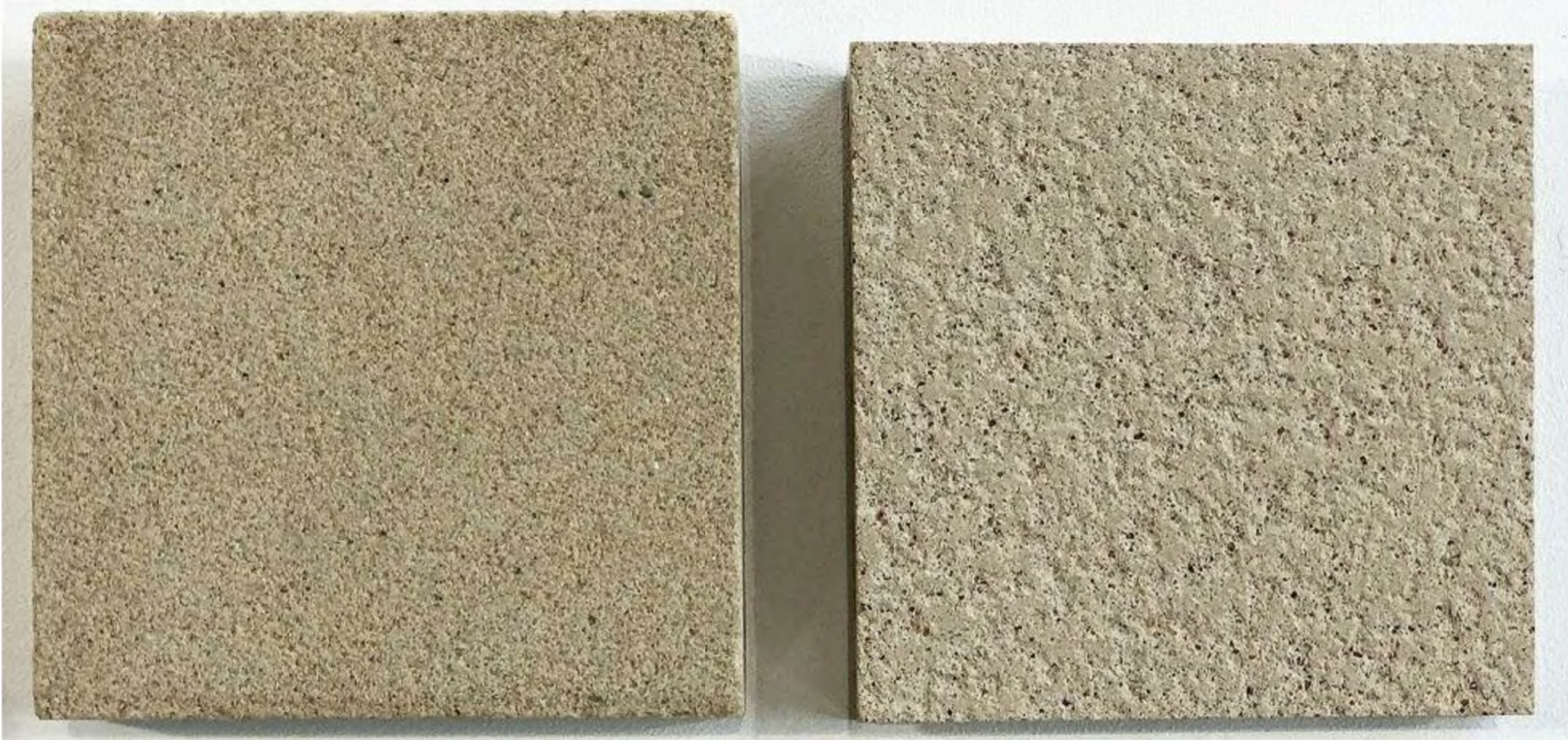
STONE WALL CLADDING, SYDNEY SANDSTONE, COLOUR CREAM (GROUND UP TO LEVEL 07. FOR MATERIAL DISTRIBUTION REFER TO DETAIL ELEVATIONS BELOW.)
