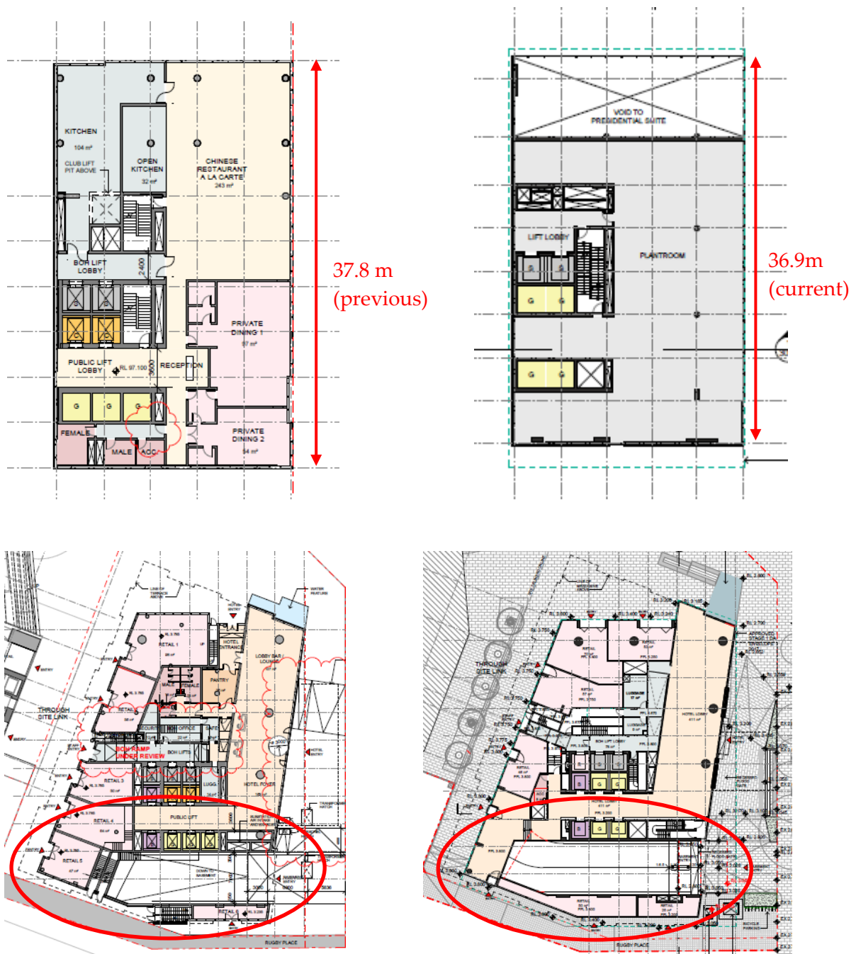
Figure 3: Tower B: Comparison of tower geometries (T) and Ground floor general arrangement (B)
