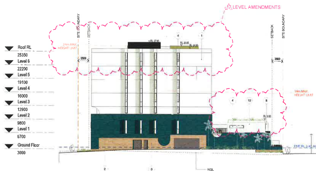
3 BUILDING B EAST ELEVATION 0201 1:250
