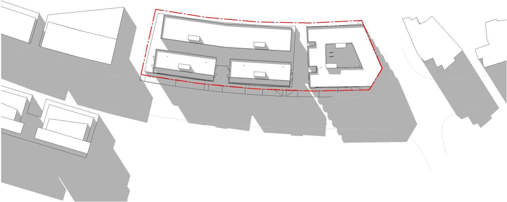
COMPLIANT - SHADOW ANALYSIS - 3PM JUNE 21
