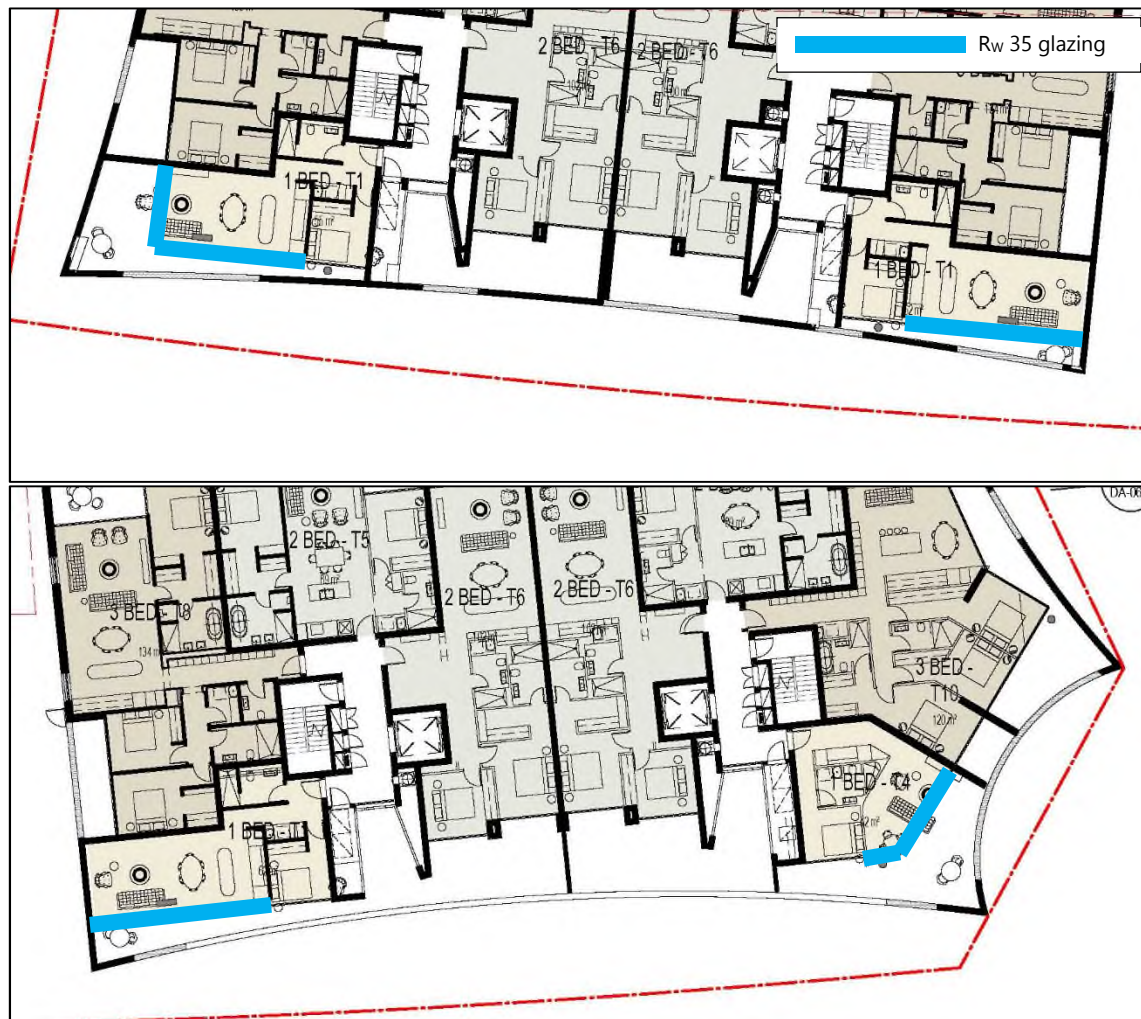
Figure 2: Mark-up of glazing requiring Rw 35
