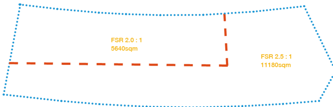
Figure 2: Maximum GFA as specified by FSR Development Standard
