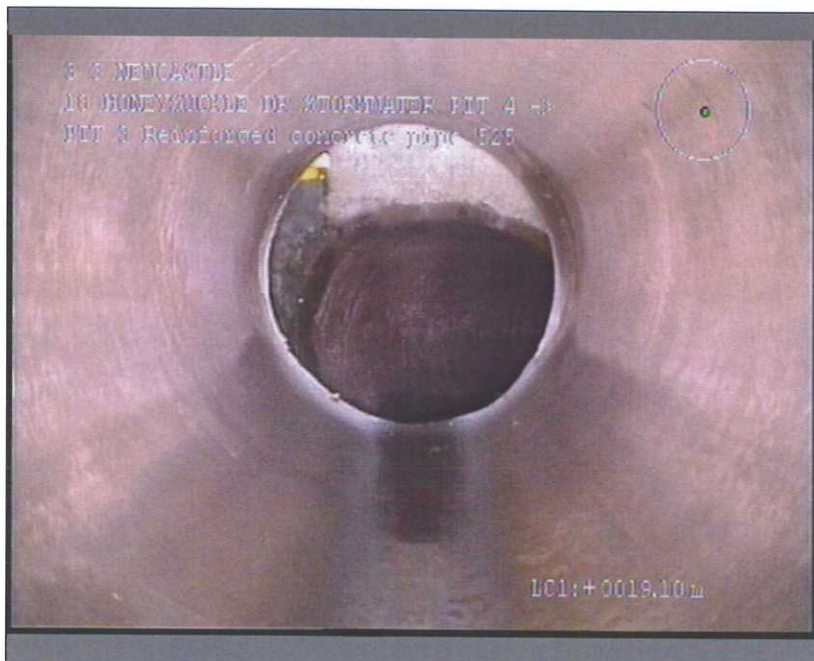
Photo: 3_4A 19.1m, Ingress of soil, fine material , at 6 o'clock, End
