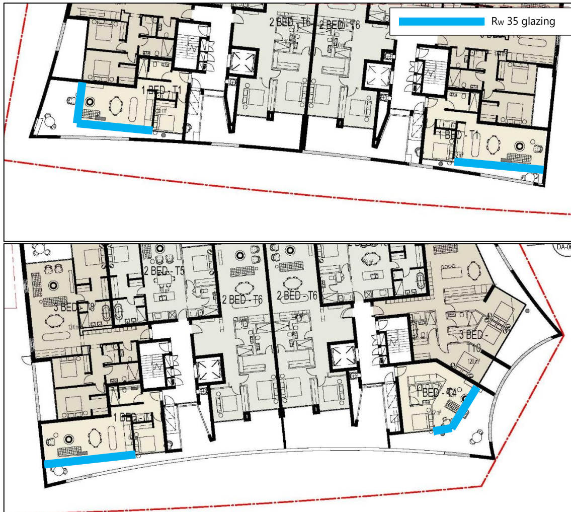
Figure 2: Mark-up of glazing requiring R_w 35
