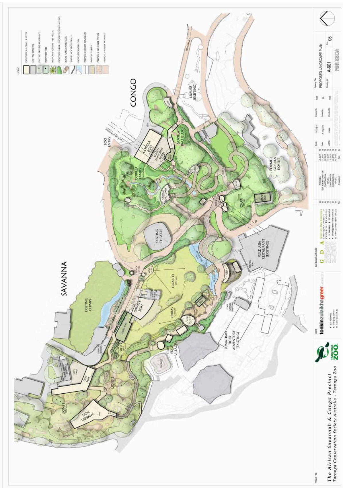
Figure 121 Proposed Landscape Plan A-601 (Courtesy Green and Dale Associates) Overall site plan indicating the extent and character of the proposed works for the new Waterhole and Congo precincts at Taronga Zoo.
