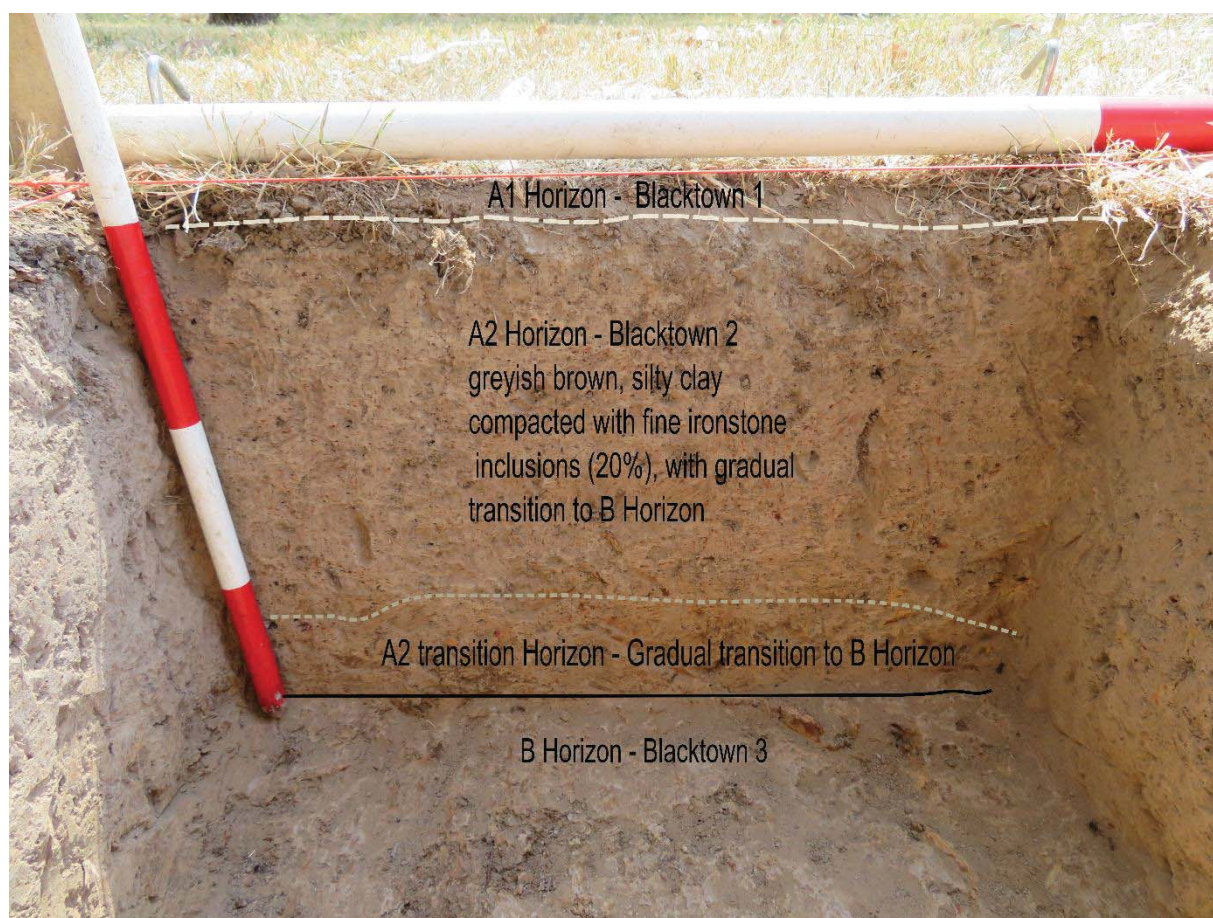
Figure 2.20 TU 34, a characteristic Type 3 soil profile—scale bar segment = 100mm. (Source: GML, 2017)
