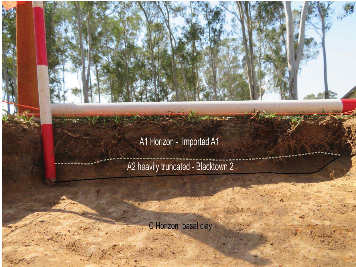
Figure 2.21 TU 40, a characteristic Type 4 soil profile—scale bar segment = 100mm. (Source: GML, 2017)
