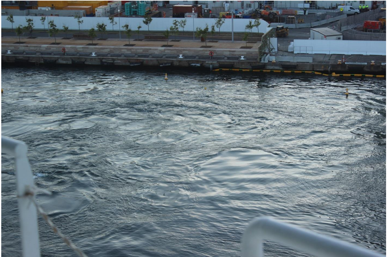
Diagram 8: Wash produced by ship's bow thruster in the vicinity of the proposed jetty during the swing of the Noordam arrival.
