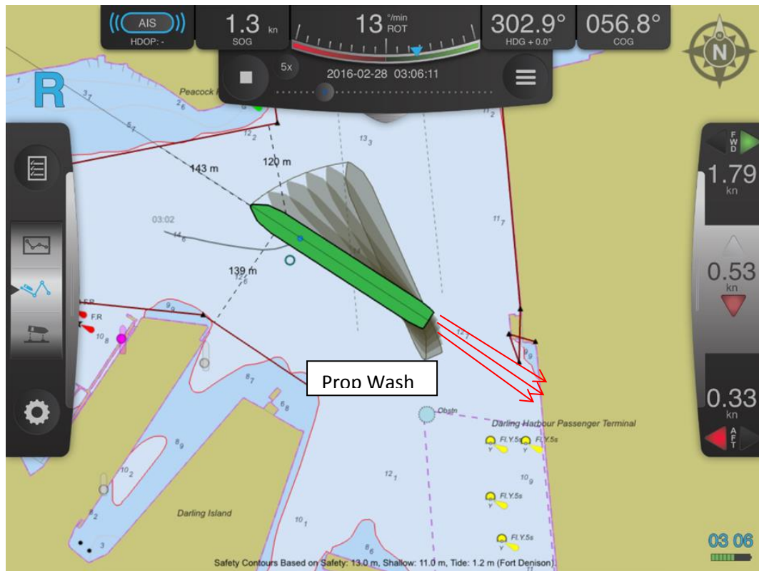
Diagram 4: Recording of vessel reversing into swing basin and indication of propeller wash as engine fires ahead
