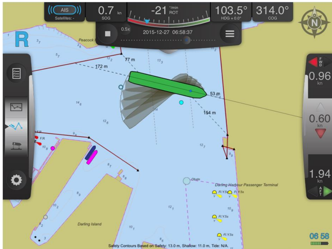
Diagram 5: Recording of arriving vessel during swing and closest points of approach to existing shoreline
