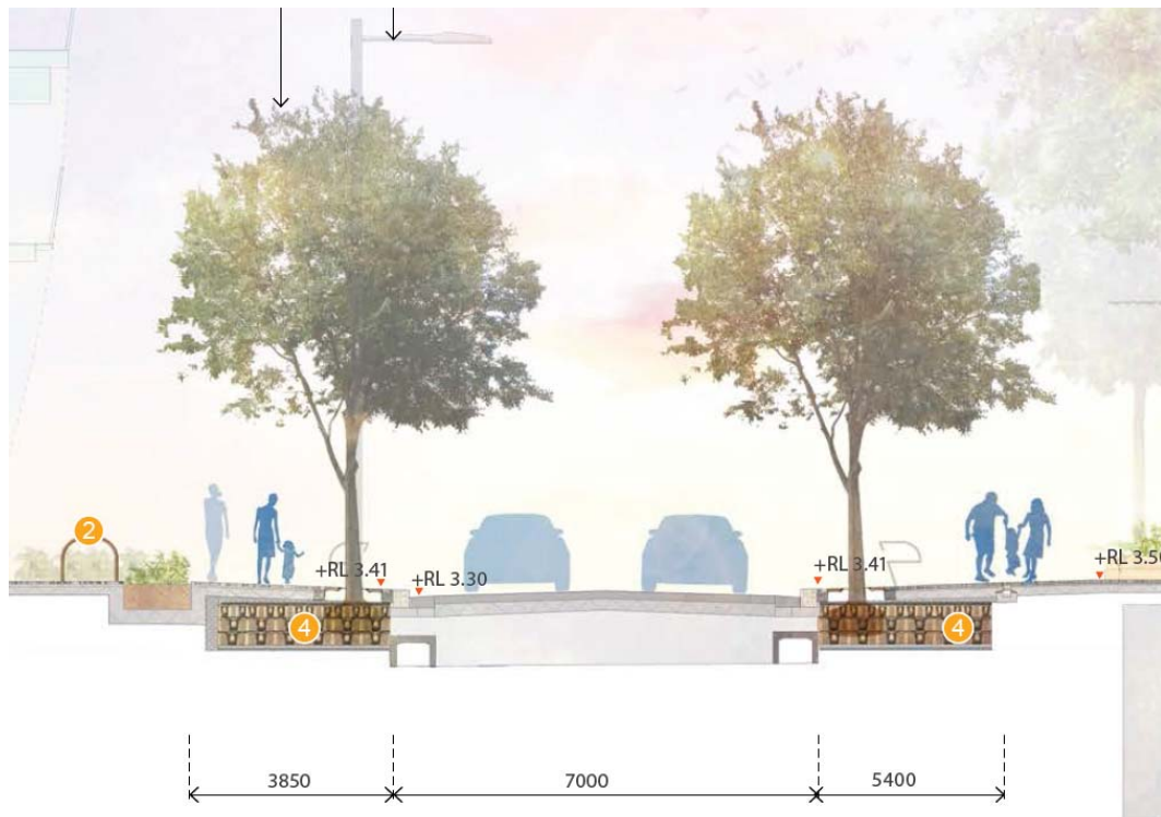
Figure 4 Barangaroo Avenue cross section
