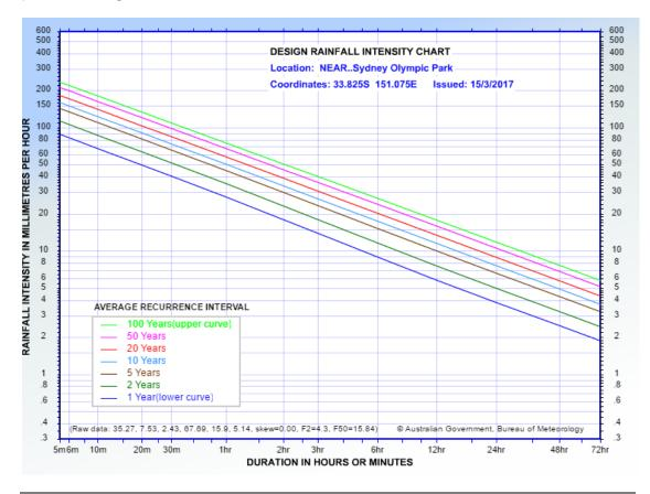
Figure 14: Intensity frequency duration chart and statistics for the site (Source BoM, 2017)
