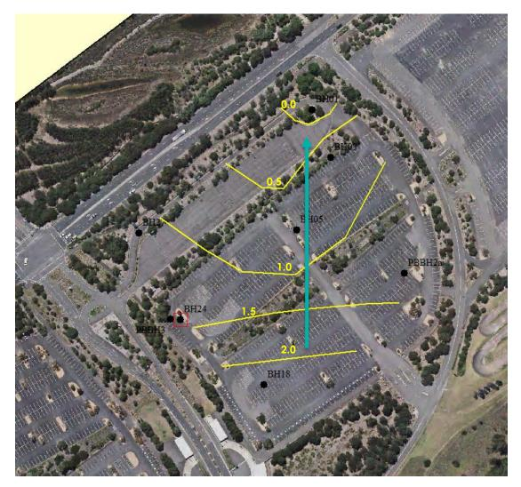
Figure 5: Groundwater levels and direction of flow
