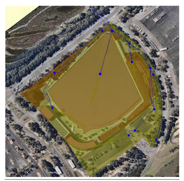
Figure 7: Modelled post-development drainage system
