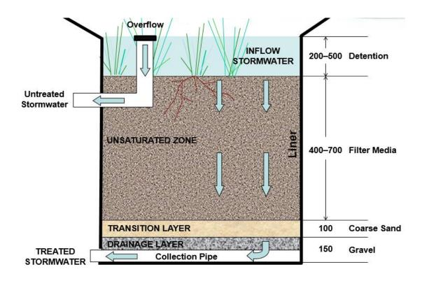
Figure 9: Typical bioretention area
