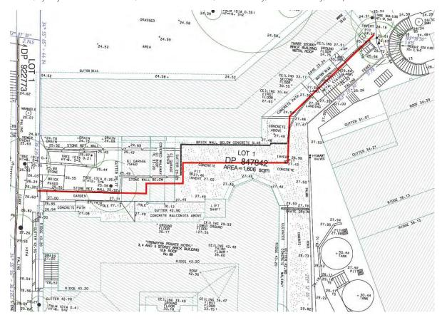
Figure 3.16 A recent survey of the area showing current location of retaining walls near B-Block. The red lines are the retaining walls on the 1890s block plan overlayed over the survey, which can be seen to closely correspond to the location of existing sandstone retaining walls. (Source: Hammond Smeallie and Co Pty Ltd, Plan Showing Detail and Spot Levels Taken Over Lot 1 in DP 847842 & Lot 1 in DP 922773 Tremayne Private Hotel, dated 10 September 2009, with GML overlay)
