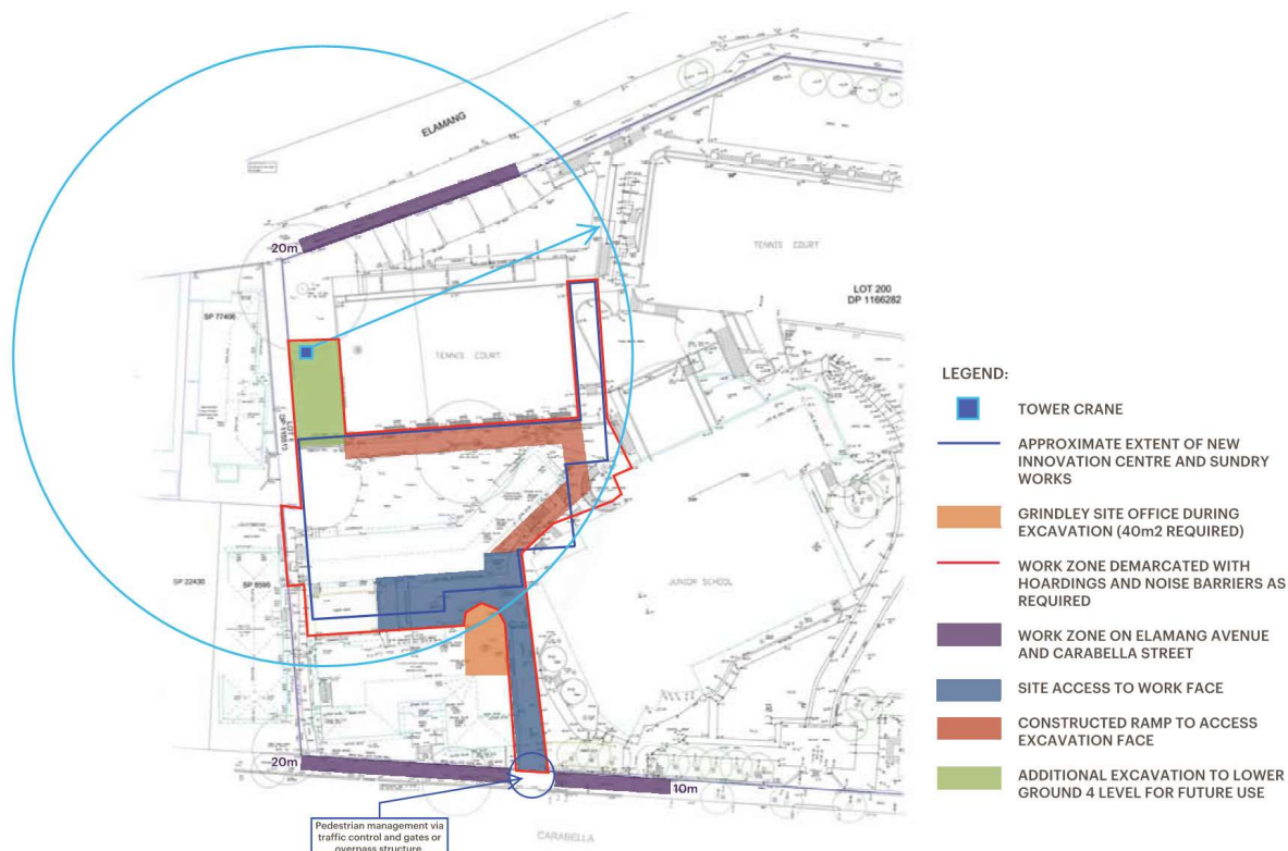
Figure 3. Establishment plan for works during earthworks, excavation & shoring. [Plan prepared by Grindley Constructions].
