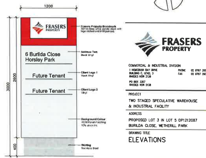
01 PYLON SIGNAGE DETAIL NOT TO SCALE
