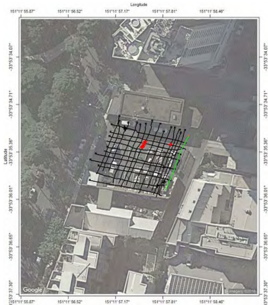
Figure 3: Plan view of the data coverage within the carpark area. Red markers indicate areas where anomalies were detected that may indicate tank like features.
