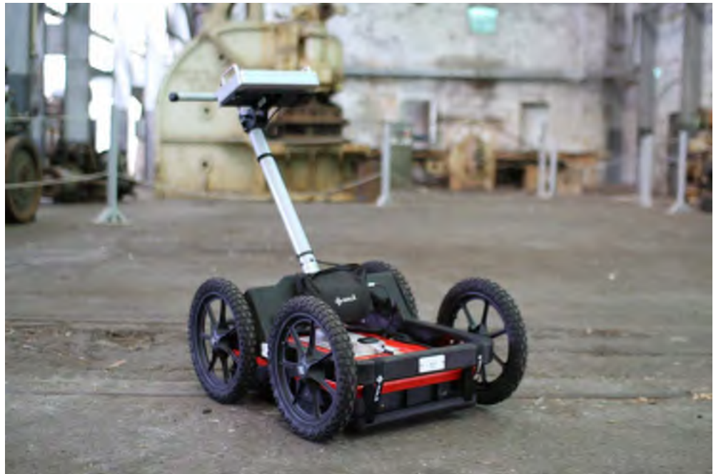
Figure 2: MALA Easy Locator HDR Wide Range GPR used for acquisition.
