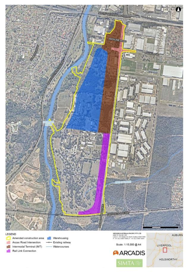
Figure 3 Key operational components
