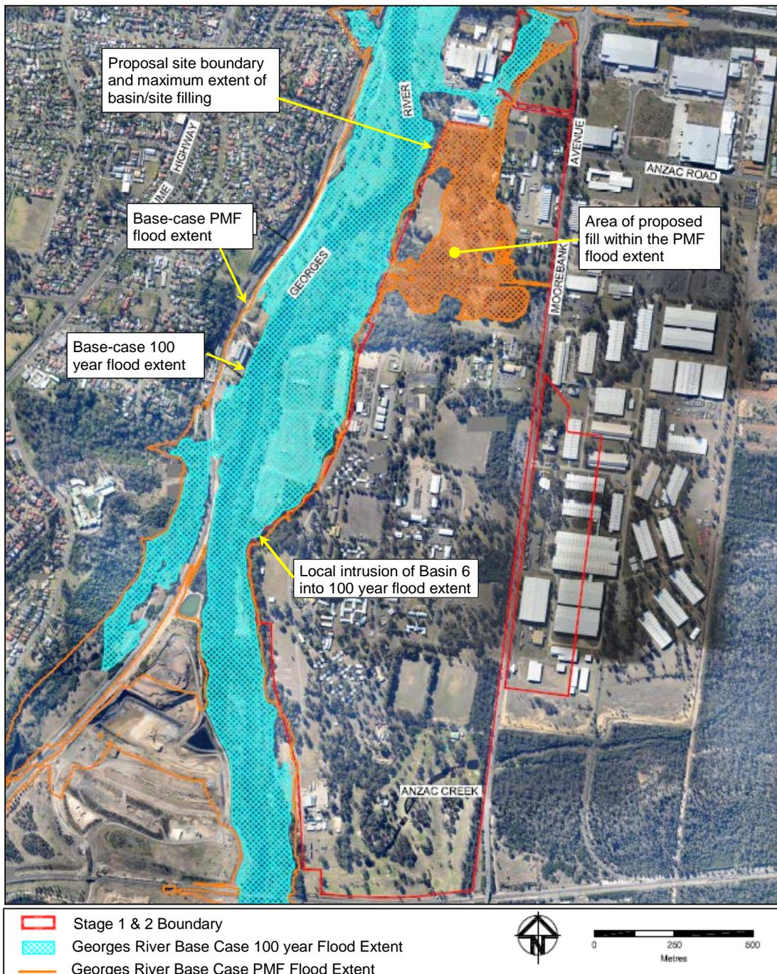
Figure 4-1: MPW Stage 2 Site Raising (Basins/Site filling) within the Georges River PMF Extents
