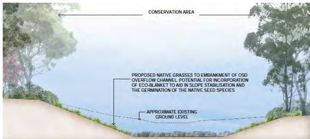
Figure 9-2 Indicative cross-section of the proposed basin outlets (adapted from GroundInk 2016)
