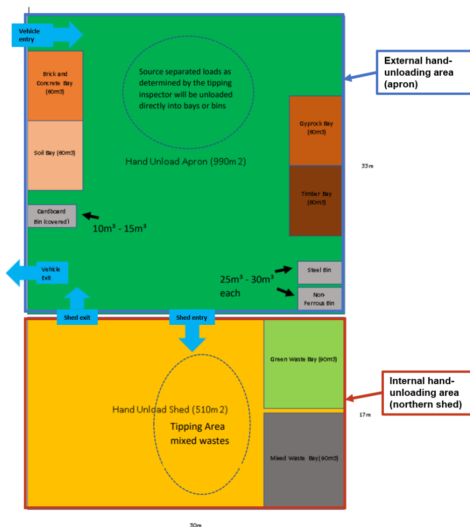
Figure 4 | Conceptual layout plan for proposed internal and external hand unload areas
