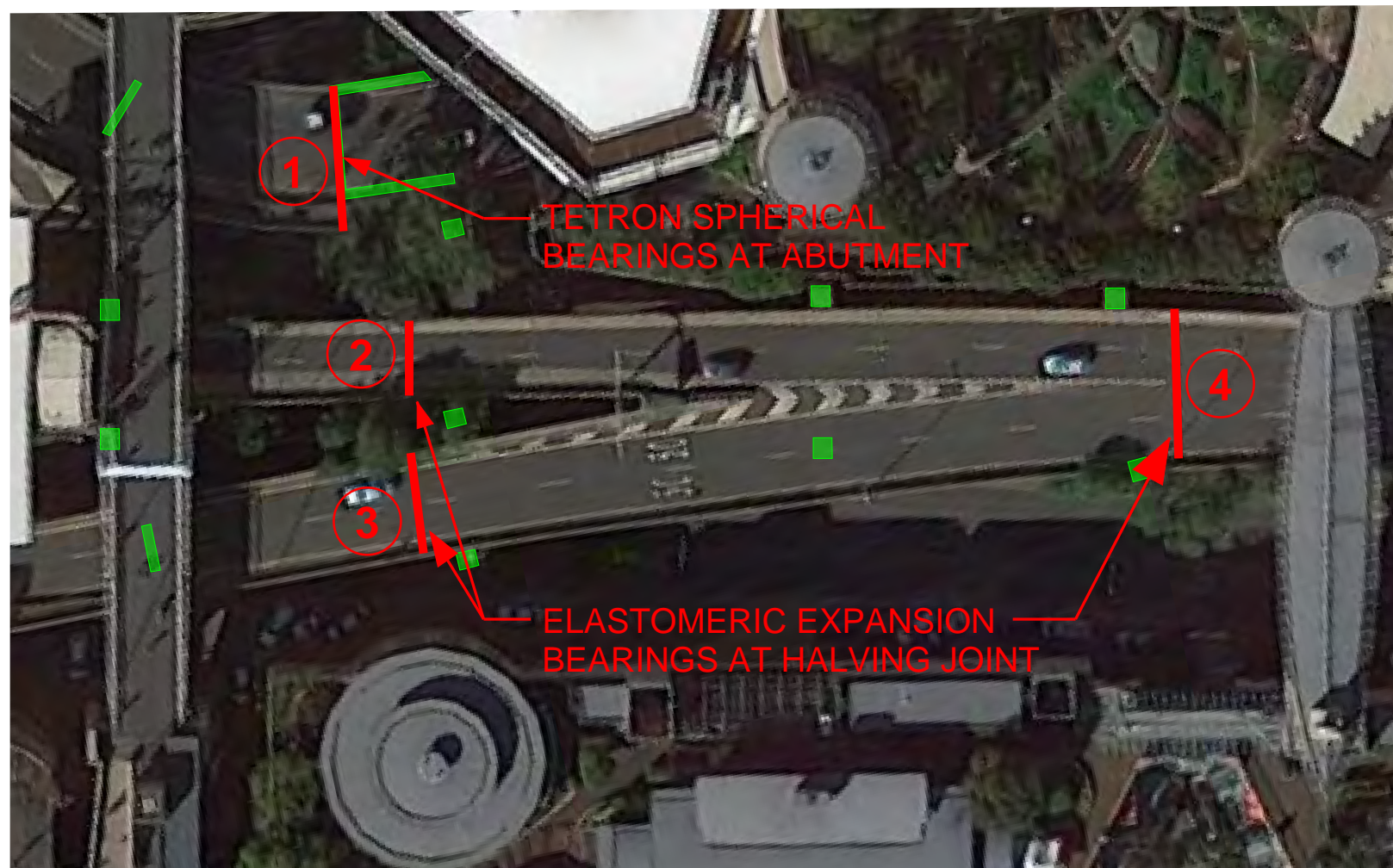
LOCATIONS OF JOINTS IN THE WESTERN DISTRIBUTOR ELEVATED STRUCTURE OVER THE EXTENT OF THE PROPOSED COCKLE BAY WHARF LANDBRIDGE
