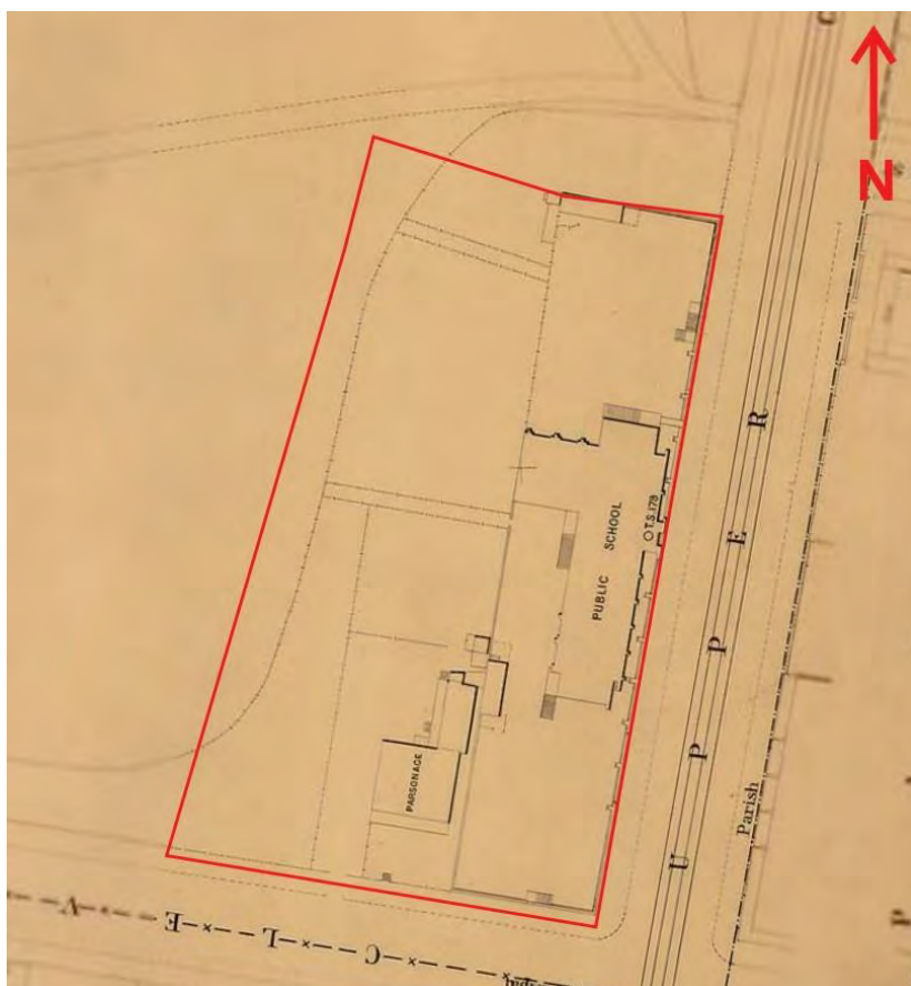
Figure 2.4: This 1886 plan of the site (outlined in red) shows the 1868 school structure. The building in the centre-south of the study area is the Wesleyan Parsonage. 'City of Sydney, Section J2, 1886', Sydney detail sheets, Surveyor-General's Office, NSW, SLNSW.
