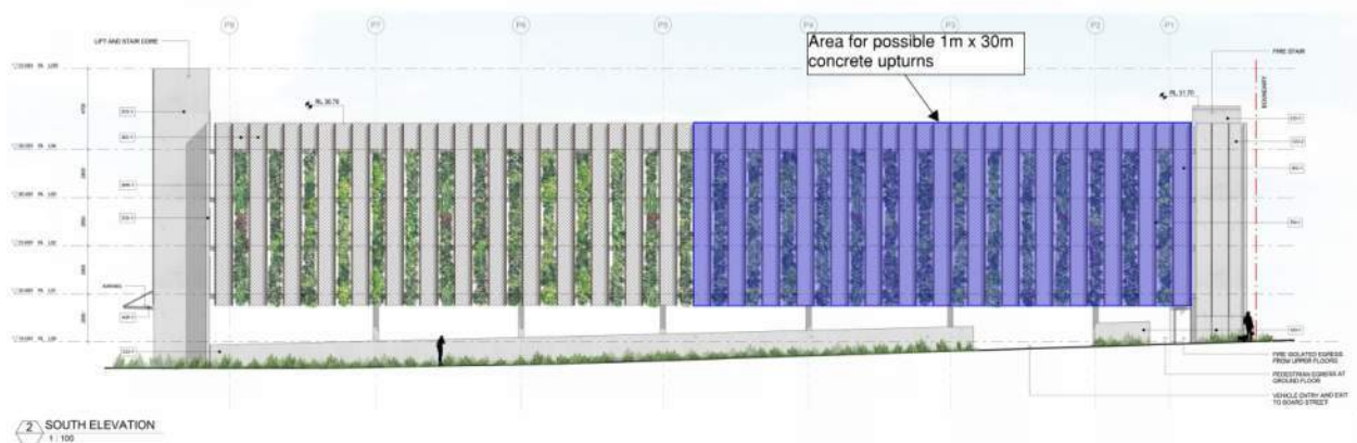
Figure 5: Southern Façade Noise control measures: 1m x 30m concrete upturns
