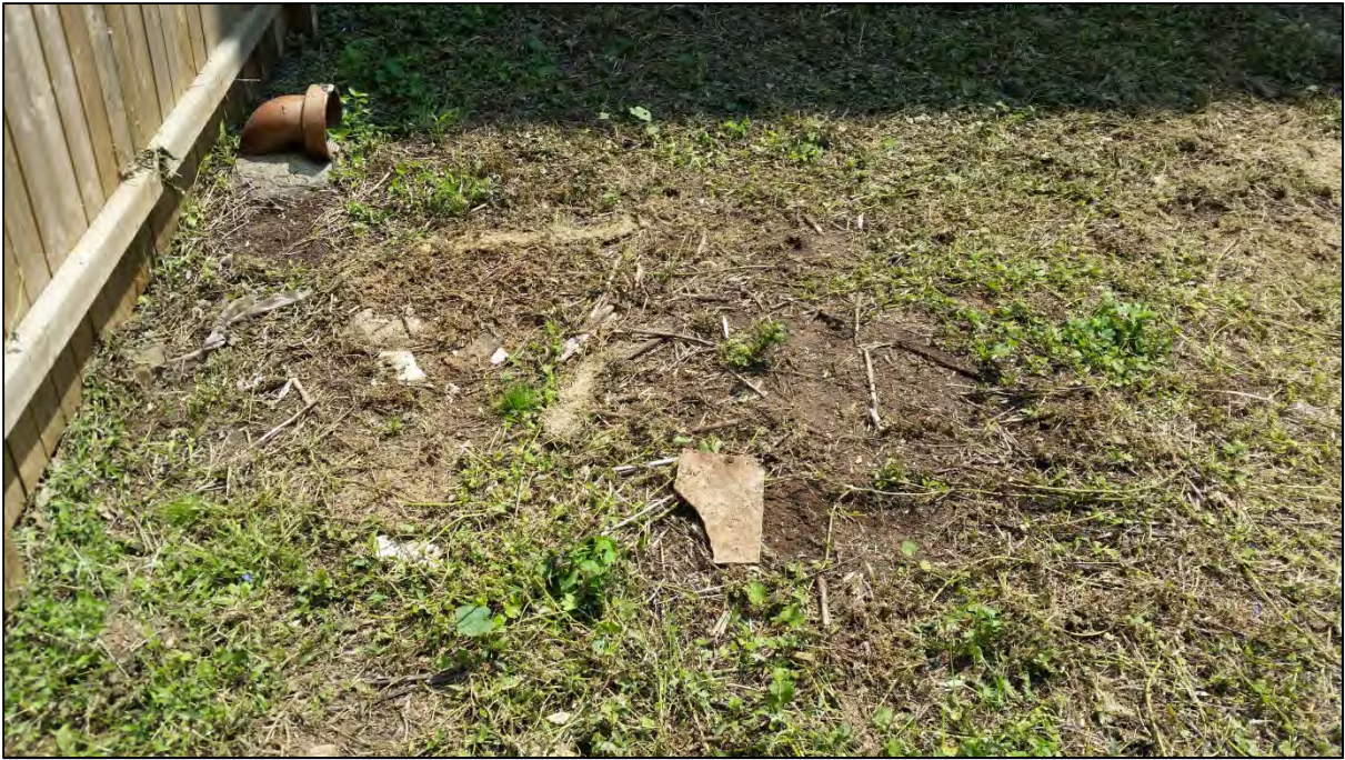
Photograph 3. Fragments of cement sheeting suspected to contain asbestos. Fragments present on surface soil of rear yard of no.26 Board Street.
