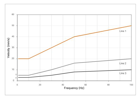
Figure 2 – DIN4150 Structural Vibration Safe Limits
