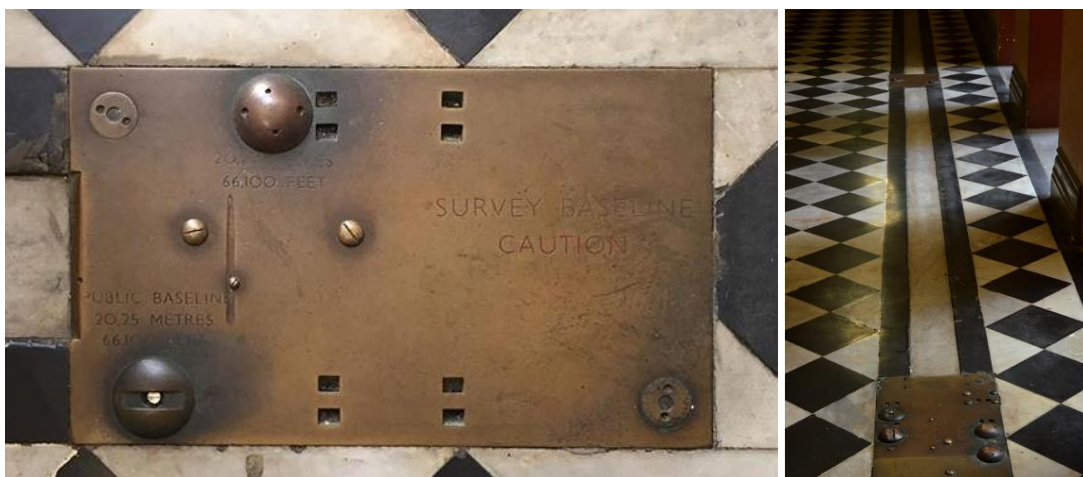
Figure 24: Baseline (top) right) on the Ground Floor, which is accompanied by a channel carved in marble which is the standard for calibrating a chain length measurement (Photo M Betteridge 2013)
