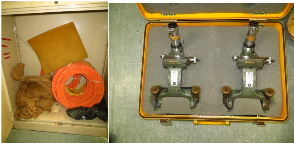
Figure 26: Chain, steel bands and surveying telescopes stored in the Lands Department Building (Photo M Betteridge 2013)
