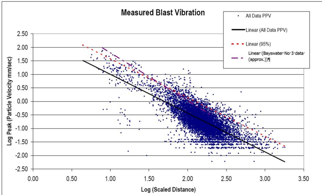
The figure shows a revised best fit line, a 95 percentile line, and also the previously-adopted 95 percentile based on 1999 data from Bayswater No 3. The correlation with the old data is close, although the new 95 percentile shows slightly lower vibration levels at shorter scaled distance – in the order of 0.2 to 0.3 millimetres per second (mm/s).
