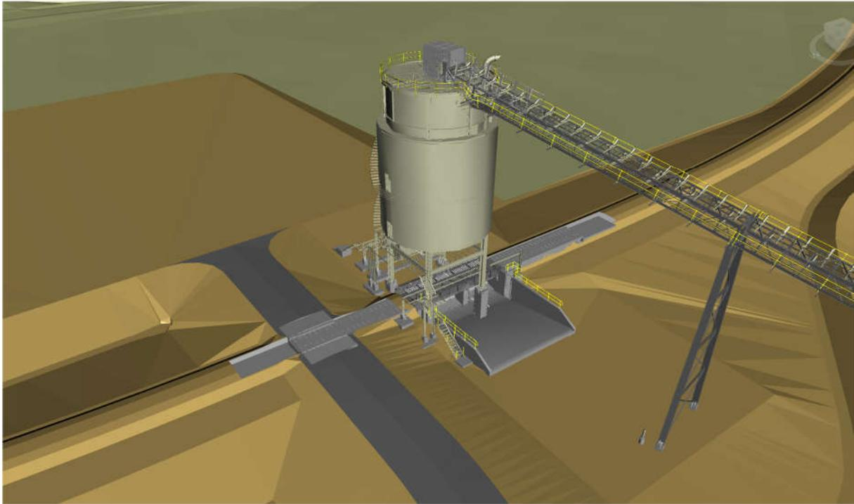
Conceptual Illustration 5: TLO Bin, Loadout Conveyor, TLO Sump and Rail
