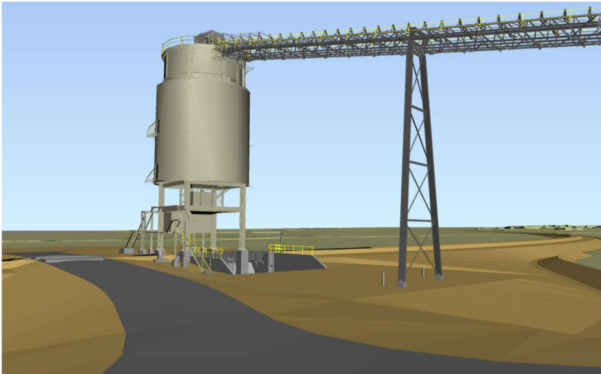
Conceptual Illustration 4: TLO Bin and Loadout Conveyor
