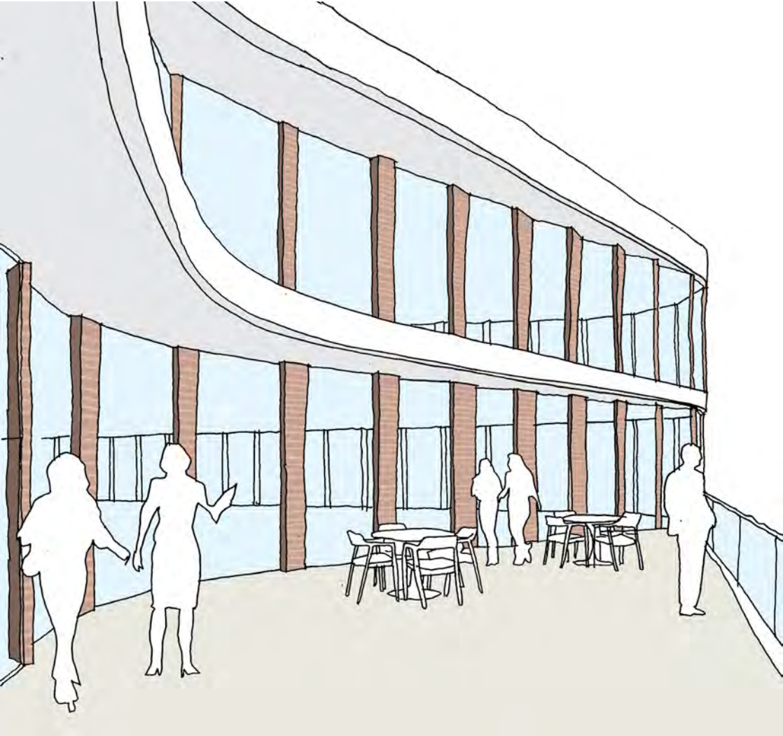
EXTERNAL TERRACES The façade curves inward at key locations to provide outdoor terraces. The large north facing terrace on level 7 is located alongside the staff breakout area and can support outdoor meetings or breakout activities. The slab projects beyond the façade line to provide weather protection and shading.
