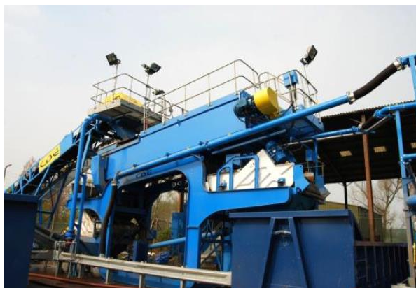
Figure 7: Example of Hydro-Excavation and Drill Mud Processing Equipment
