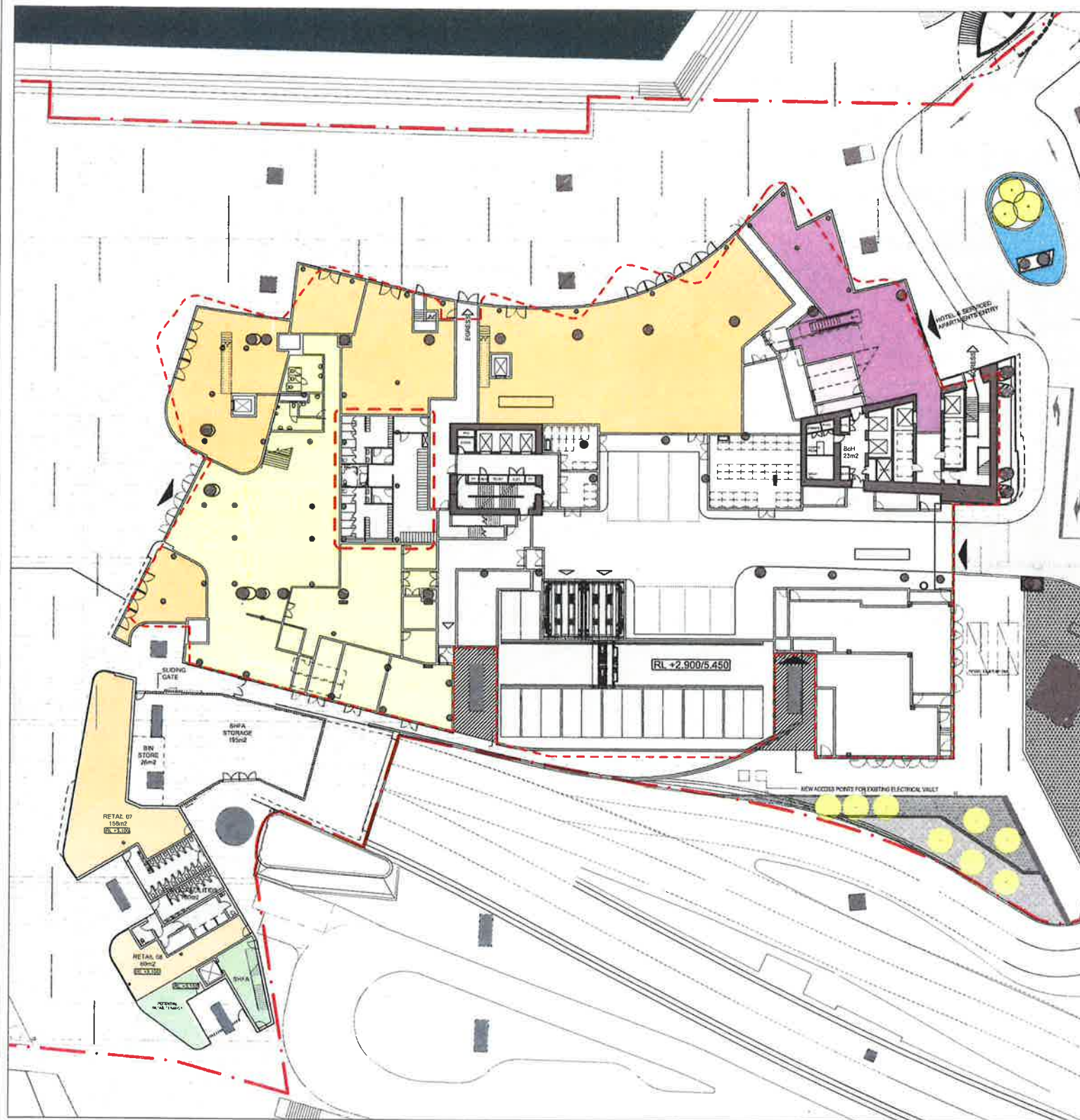
1 GROUND FLOOR PLAN - LOCATION OF CLASS B BICYCLE PARKING AND END-OF-TRIP 1:250
