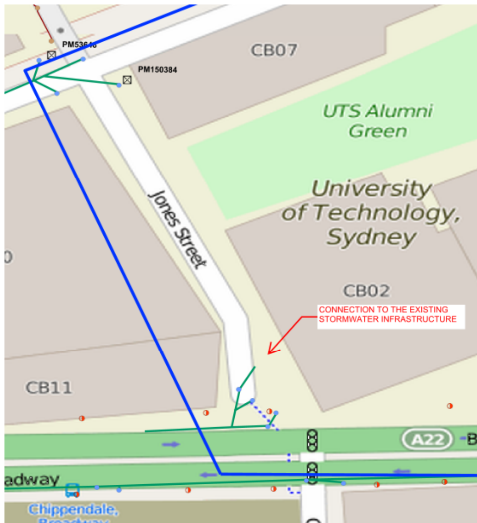
Figure 1 This plan indicates the existing sewer and storm water connections, including sewer infrastructure. This information is based on existing UTS drawings and information provided by Sydney Water. The infrastructure shown above is the property of Sydney Water.
