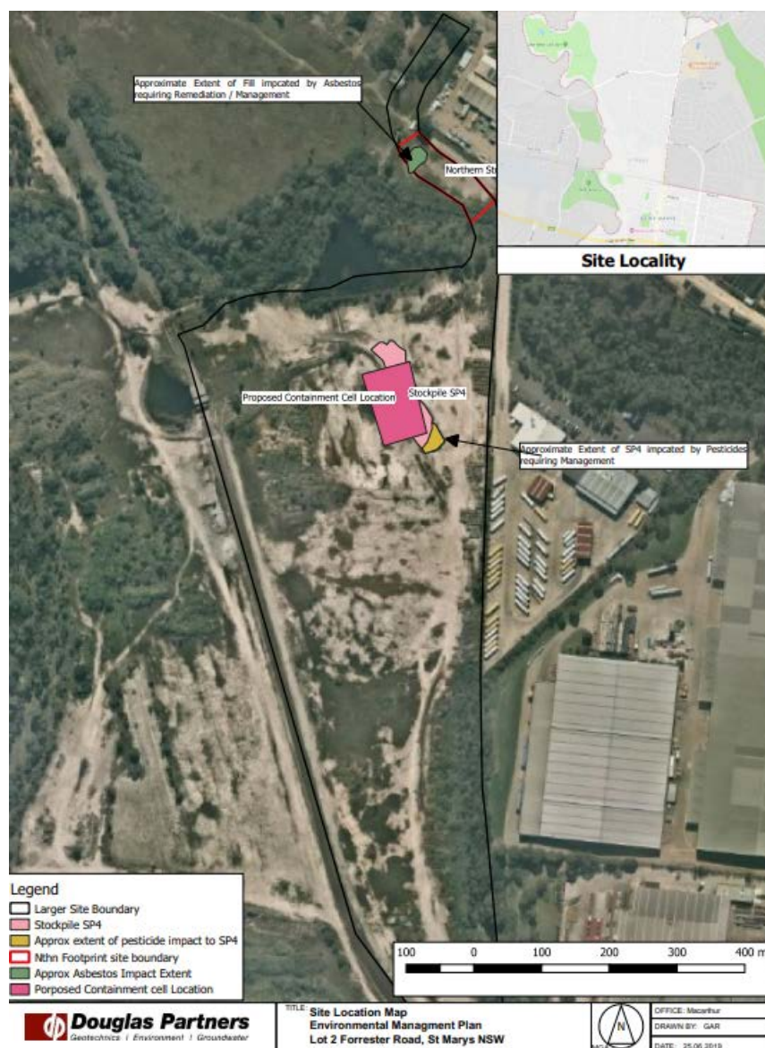
Figure 12 | Site Location Map, showing extent of contamination to be remediated (Source: Interim Environmental Management Plan, Douglas Partners, August 2019)
