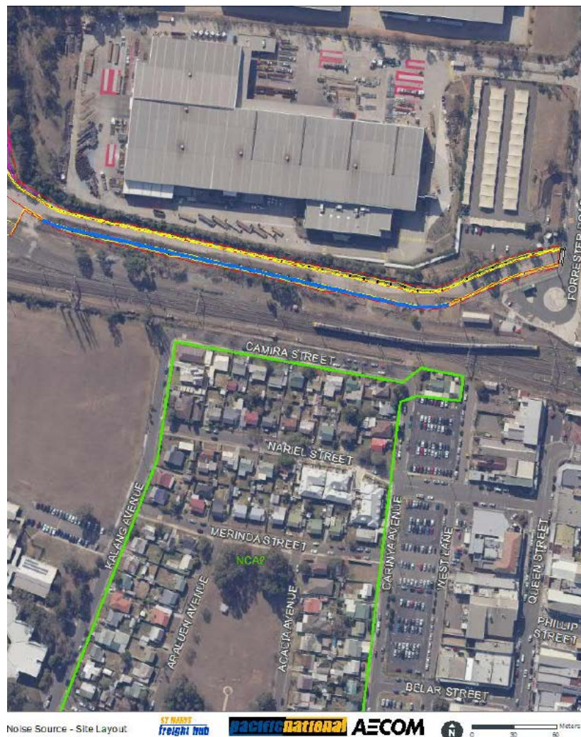
Figure 10 | Applicant's proposed noise barrier location (blue line) (Source: Figure 3 of Applicant's NVIA)
