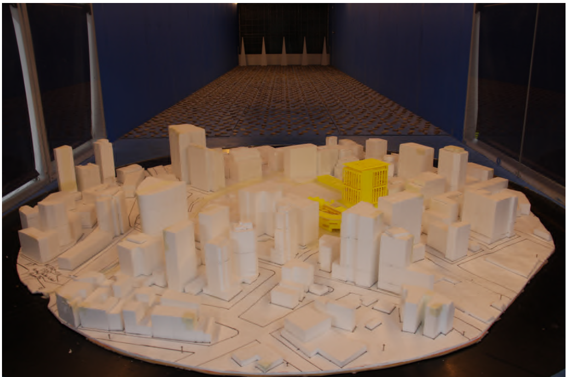
Figure 2c: Photograph of the Wind Tunnel Model – View from the South-East
