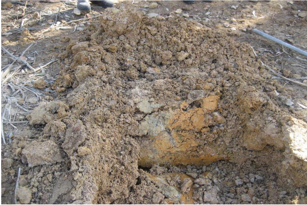
Photo 6: View of clayey material encountered during test pit excavation along leachate dam.
