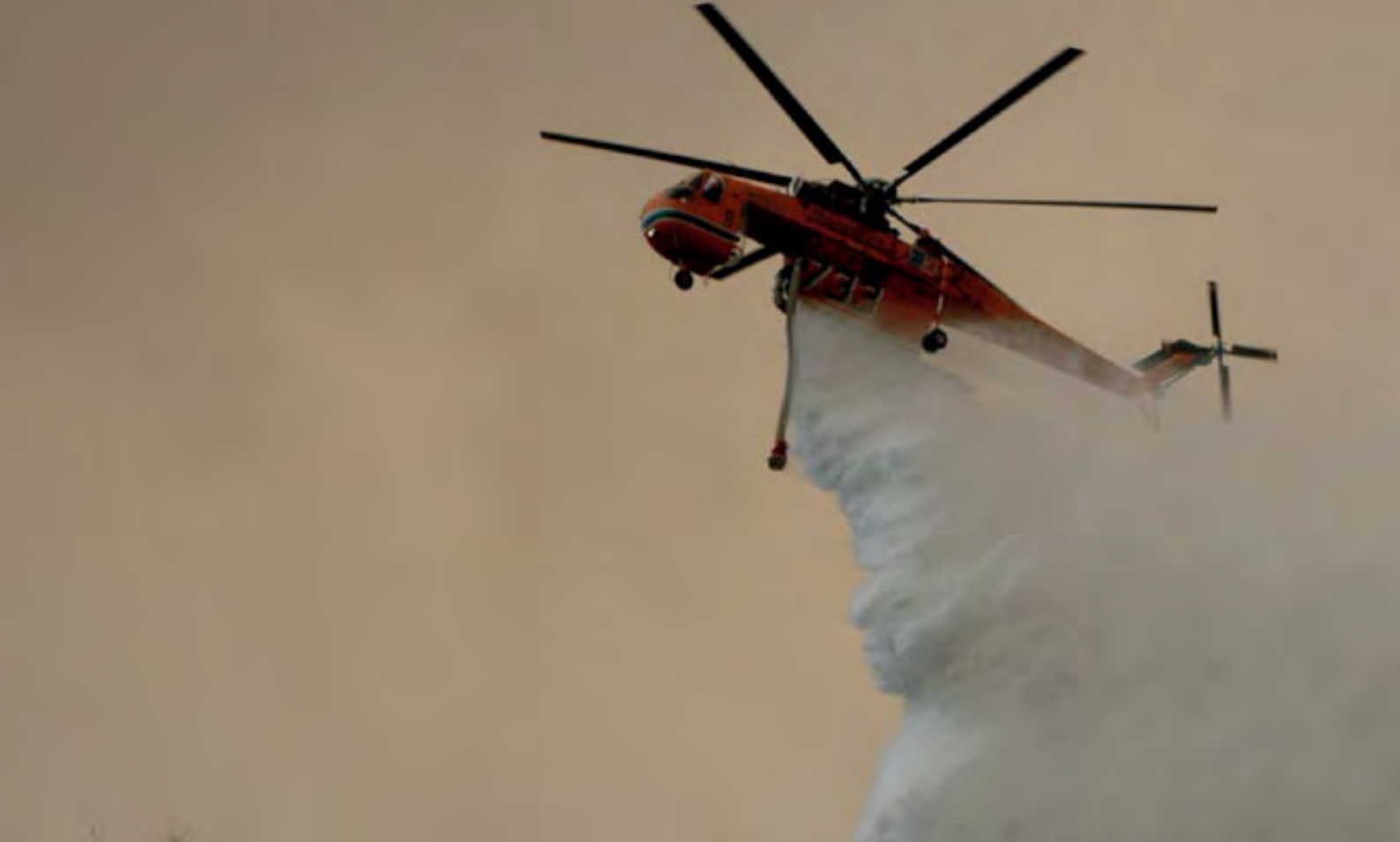
Figure 16: Elvis – the Erickson Air-Crane fire bomber – dumping about 9,000 L of water to assist firefighters battling a blaze in Australia's southeast. Specialised firefighting aircraft like this are loaned for the bushfire seasons in both the Northern and Southern hemispheres each year. Such aircraft are expensive to operate.
