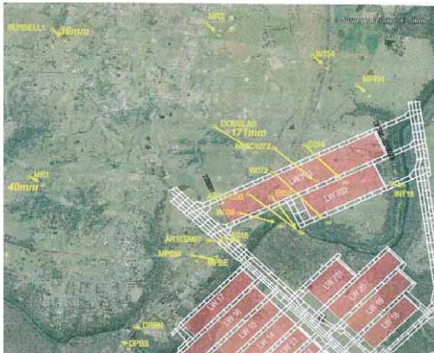
FIGURE 4.2. Measured Far-Field Movements at the Completion of LW703 (Pells 2011)
