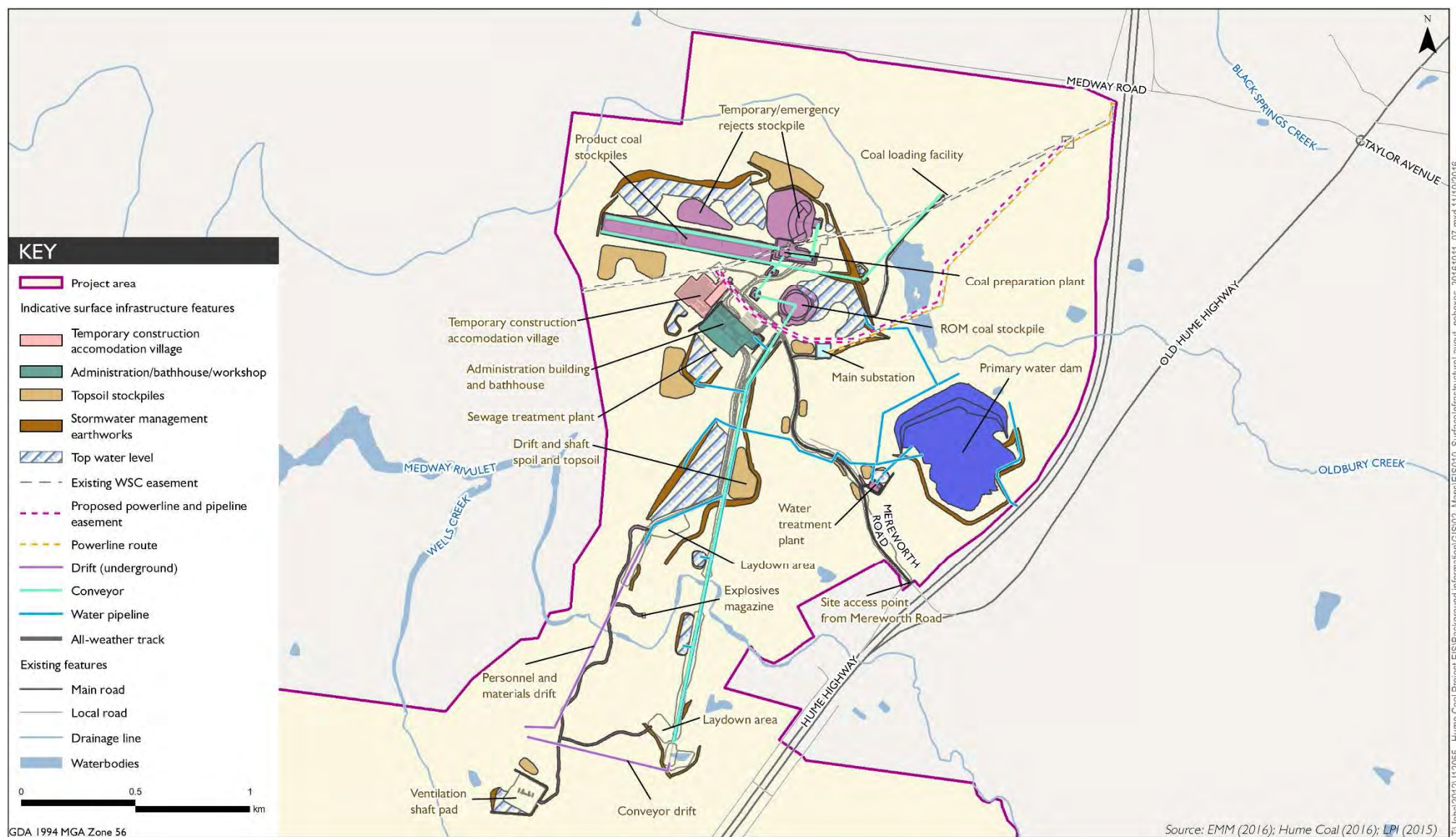
Figure 1.2. Indicative surface infrastructure layout. Coffey GEOTLCOV25281AB-ACB 17 November 2016
